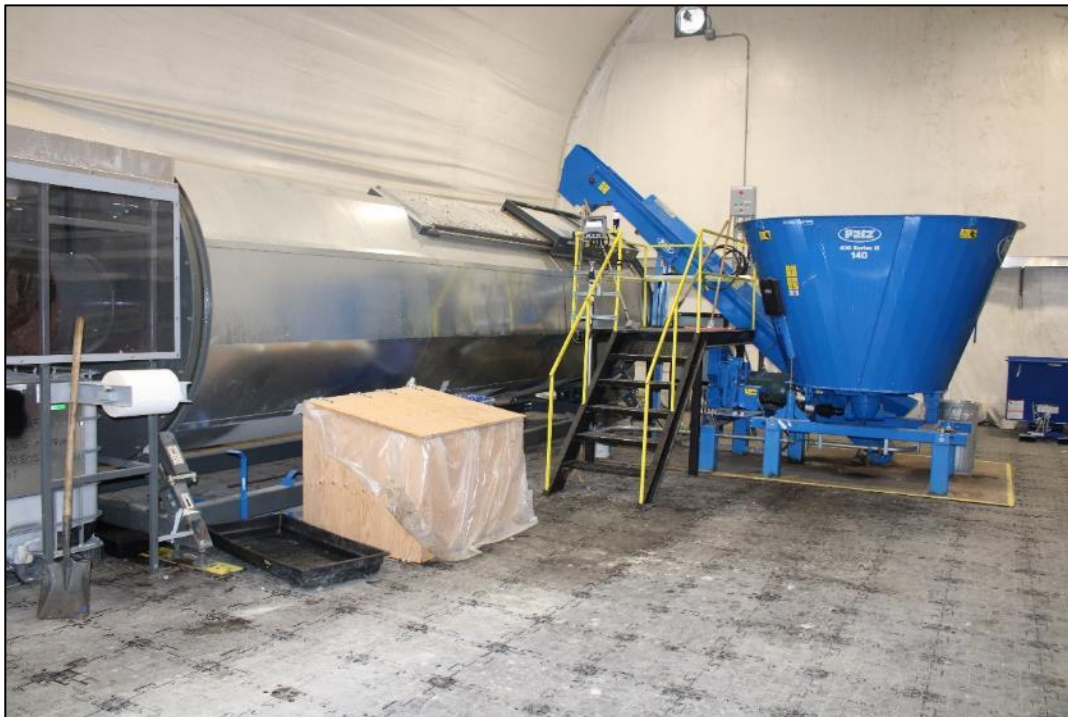
Photo 15: Industrial Composter Installed at the Incinerator Facility.
