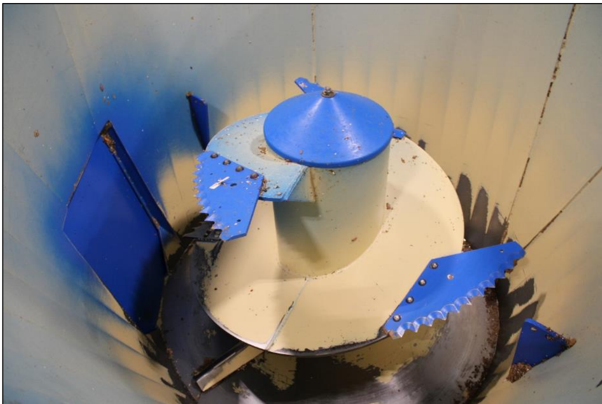
Photo 16: Hopper for Organic Waste to be Loaded.
