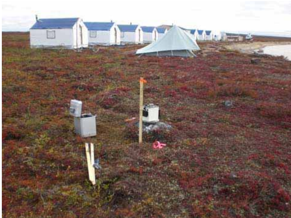
Figure 15: One of the gravity meters used by MWH Geo-Surveys Ltd. while conducting ground gravity surveys for Forum Uranium Corp.
