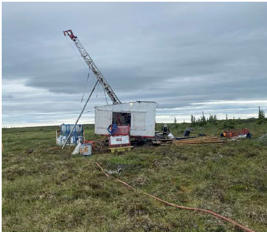
Figure 7: 2023 drilling at Lac 50 Main Zone with a Boyles 17 heli-portable rig with cuttings settling tanks.
