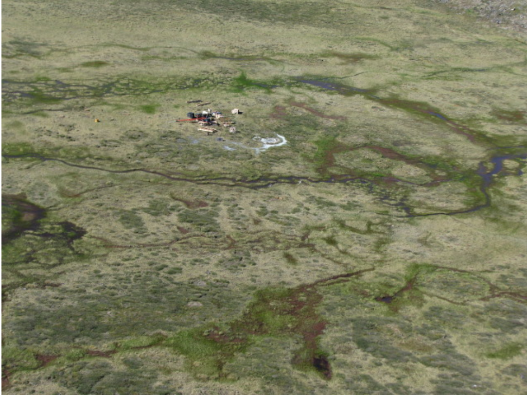
Figure 9: Typical drill hole after completion. The milky residue is mostly very fine particulate matter and biodegradable drilling additives in the drilling fluids.
