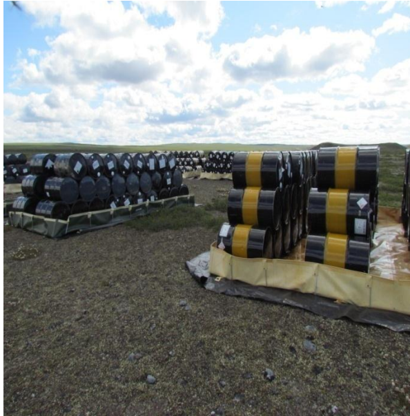
High Lake East showing fuel storage with secondary containment.
