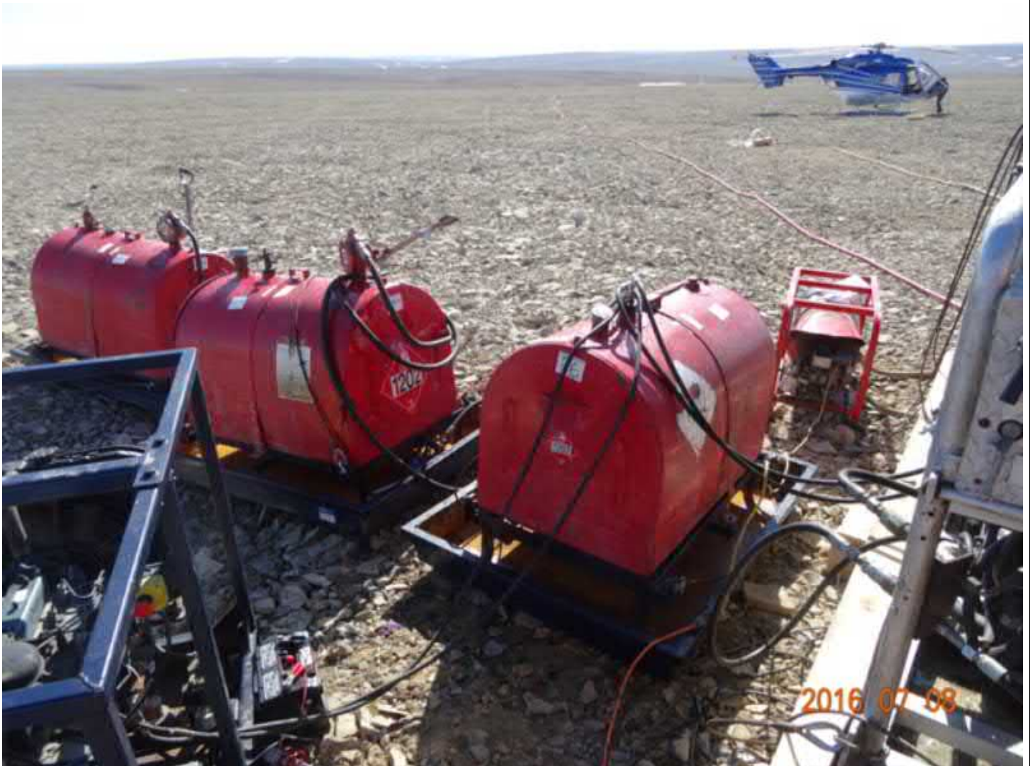
Figure 8 Fuel storage all double walled transport containers
