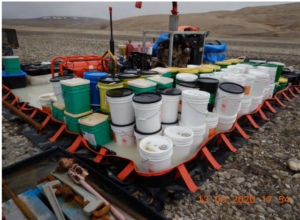
Photo 7. Photo captured by Mr. Monteith during the 2020 inspection. A 5 gallon container of non-hazardous, non-toxic drilling fluid (AMC CR 650) spilled and was contained within the berm.
