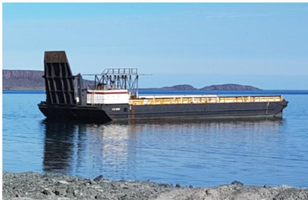
The FM 503 is a versatile ramp equipped deck barge. The barge was completely refurbished in 1998 adding a helicopter landing pad and new hydraulic bow ramp. The 503 has been utilized as a helicopter support barge, cable-laying vessel, and coastal equipment barge. She has generators and hydraulics on board as well as two large capacity pumps for the ballast system. The 503 is equipped as an oil spill response barge and has capacity to store 1500 M3 of recovered oil.
