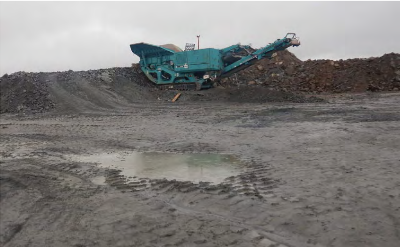
G-27. - Surface undulation of the crusher pad
