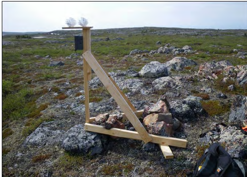
Photo 3.8-1 Remote Camera Setup using a Wooden Tripod and Security Box
