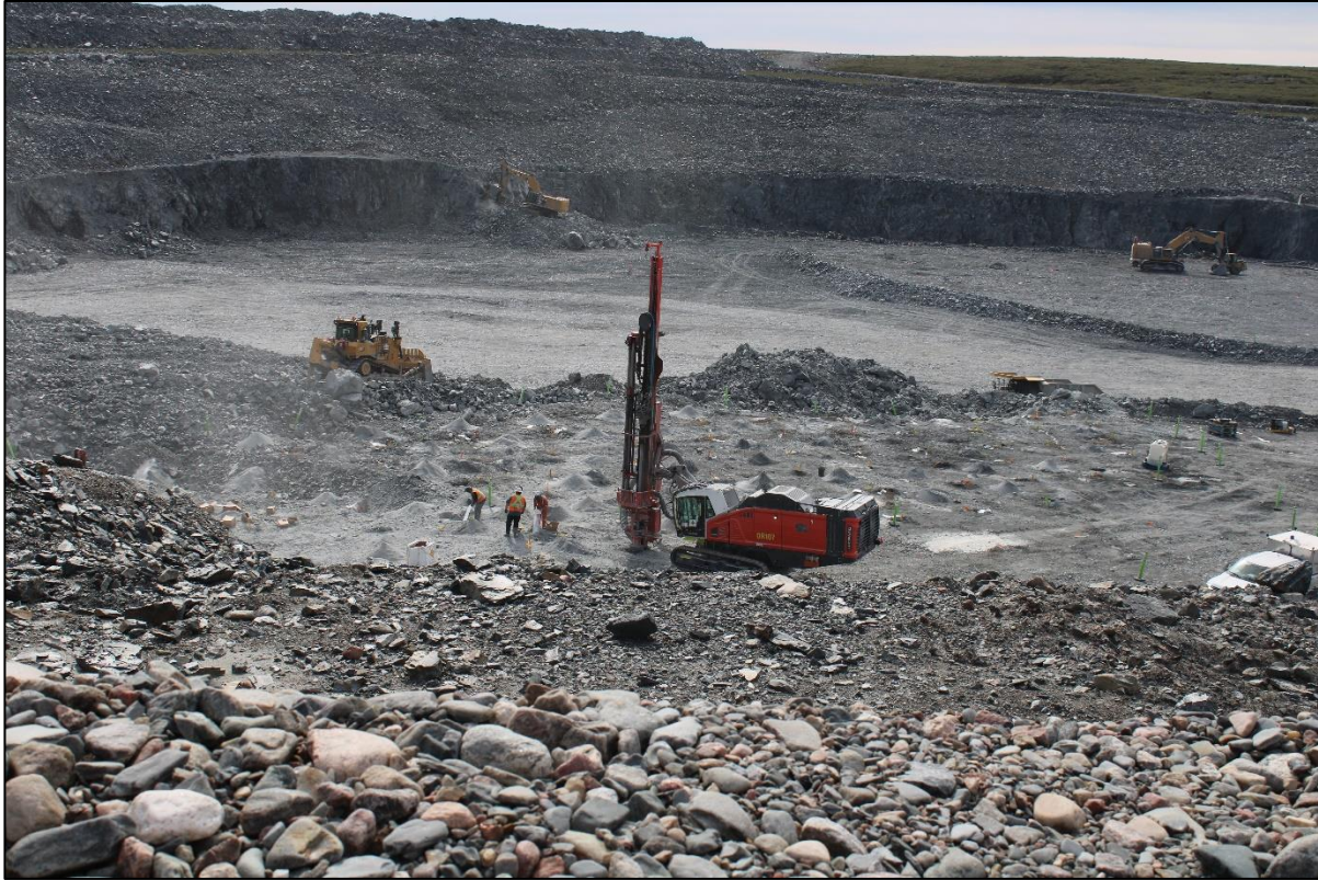
Photo 19: Blasting preparation in Echo Pit
