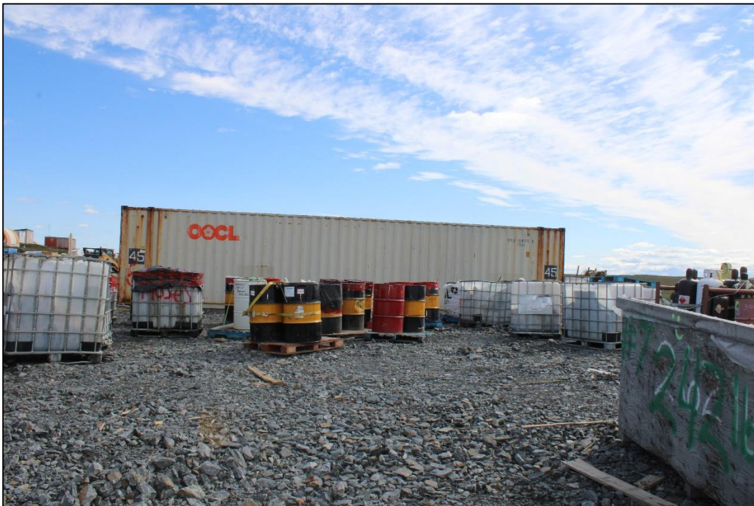
Photo 16: Hazardous Materials Stored outside of lined containment
