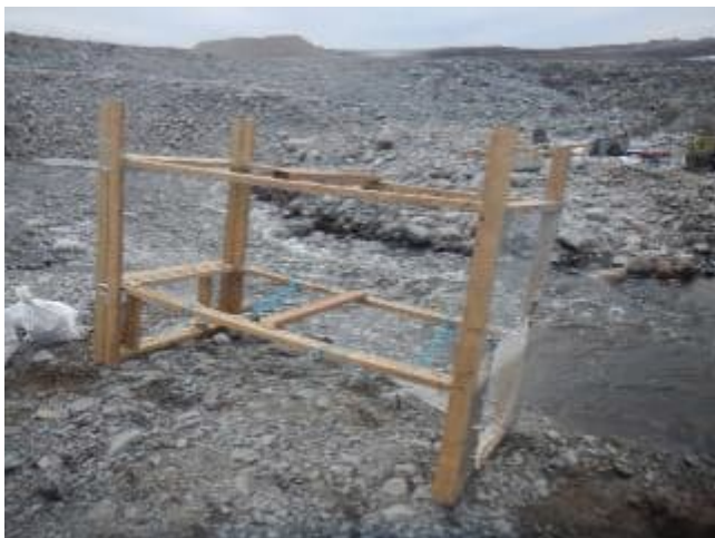
Photo B-10: Fish trap frame and funnel mouths w/o conduit.
