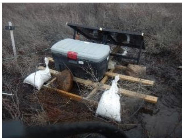
Photo B-18: Action packer with Data logger, battery and solar panel setup at RFID Array 1.
