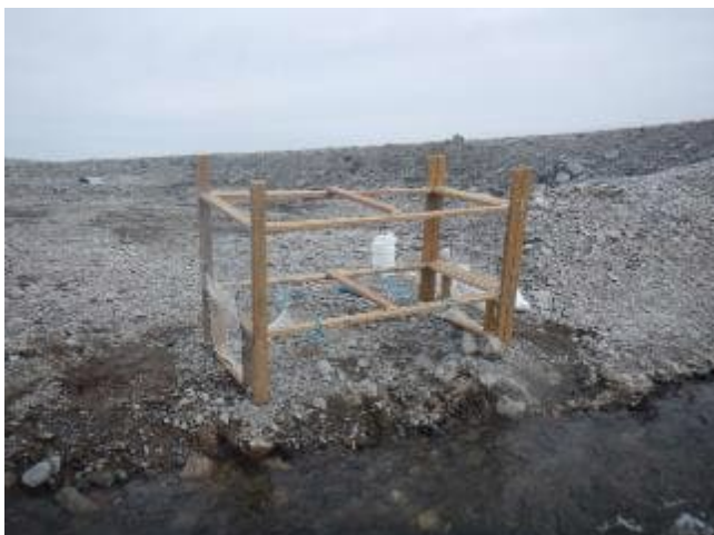
Photo B-12: Fish trap frame and funnel mouths w/o conduit.
