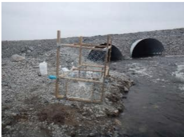
Photo B-11: Fish trap frame and funnel mouths w/o conduit.
