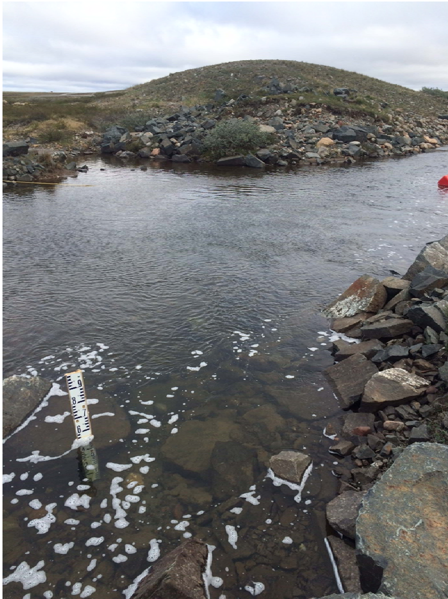
Figure 1: Staff Gauge Installed at Char River
