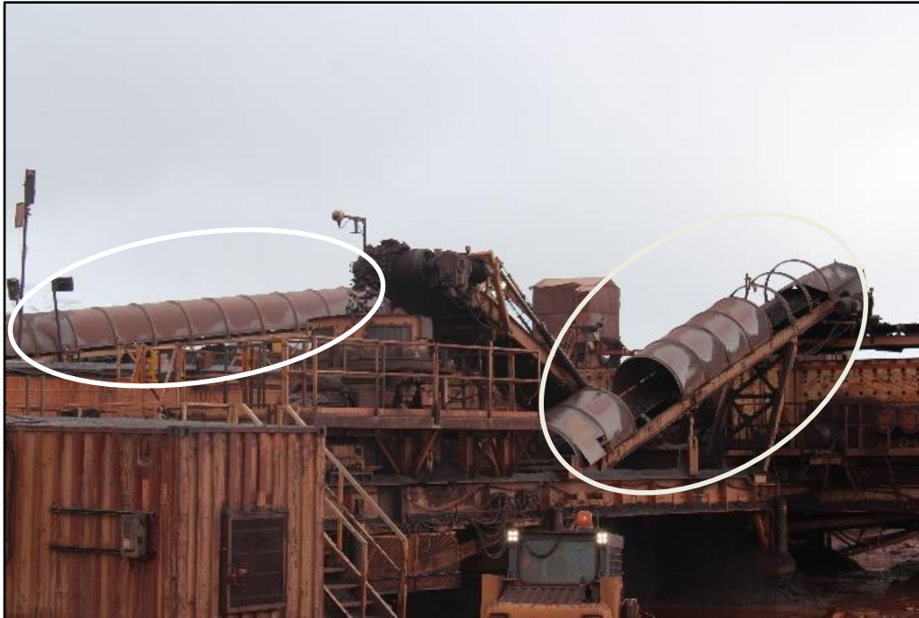
Photo 12: Hoods Present at Crusher Conveyor.
