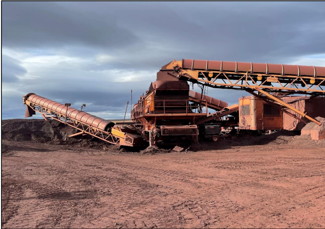
Photo 29: Example of Hoods Covering the Conveyor Belt
