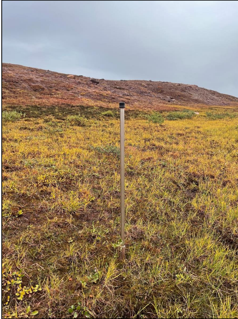
Photo 40: Groundwater Monitoring Well Next to the Landfill
