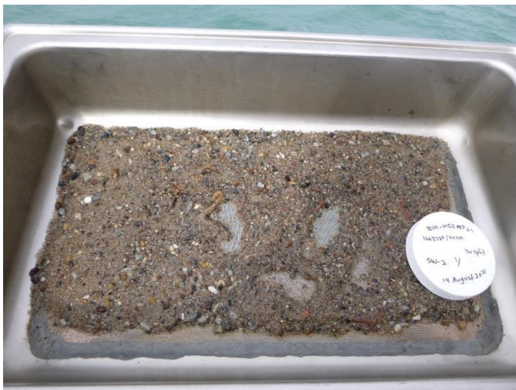
Photo 4 – Benthic sample on 0.5 mm sieve, collected at station SW-2 on 14 August 2021.
