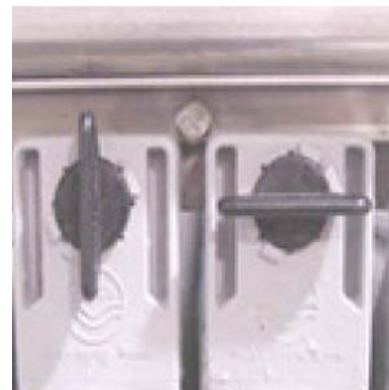
Figure 5.24 - Locked Module Key (Left)
