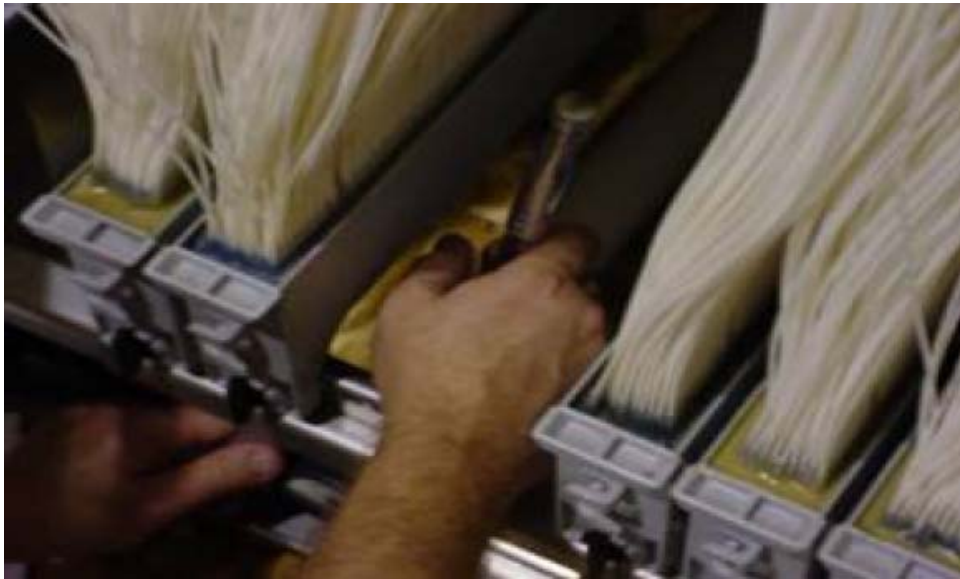
Figure 7.8 - Removing the Bolts
