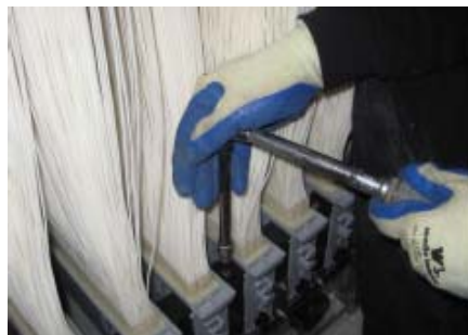
Figure 5.25 - Tightening Expanders
