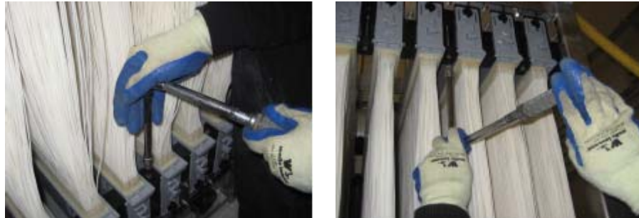
Figure 7.6 - Tightening Expanders
