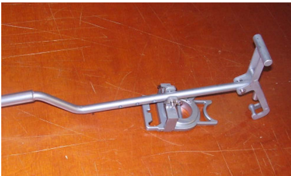
Figure 5.26 - Module Removal Tool
