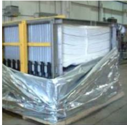
Figure 5.4 - Shipping Braces
