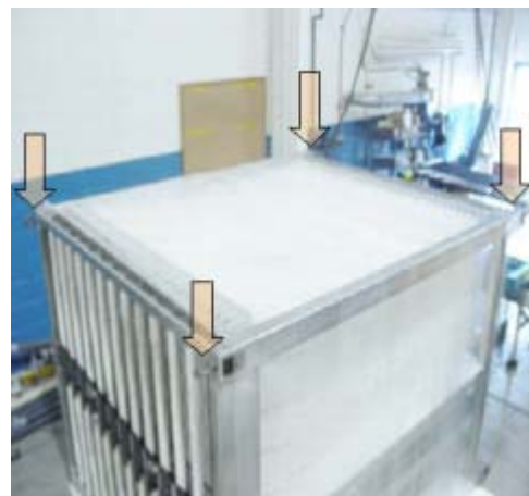
Figure 5.5 - Hoist Ring Locations
