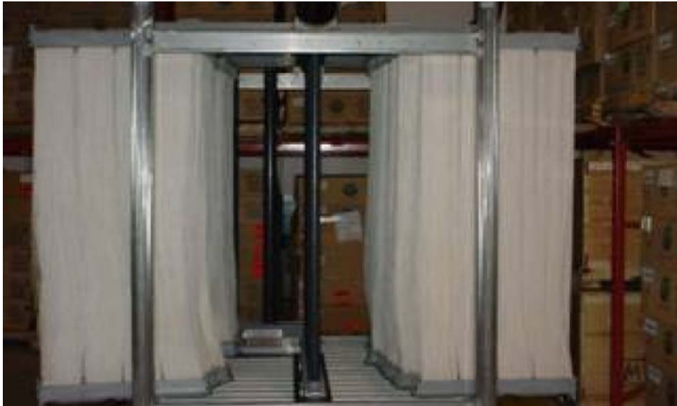
Figure 7.11 - Slide the Modules to the Stop Position
