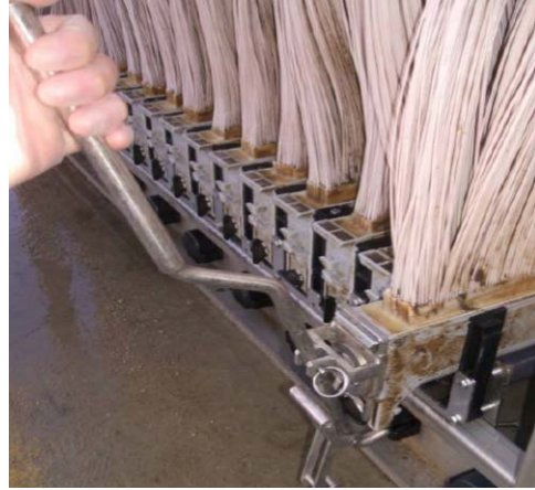
Figure 5.32 - Removing Module with MRT
