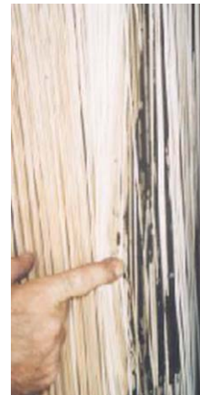
Figure 7.1 - Solids Accumulation Between Fibers
