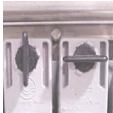
Figure 7.7 - Unlocked Module Key (Right)
