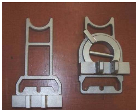
Figure 5.27 - Standard (Right) & Repair Adaptor (Left) MRT Faceplates
