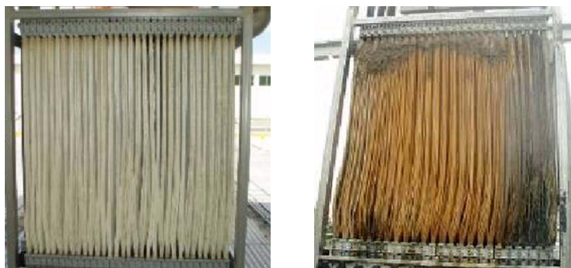
Figure 10.2 - Acceptable (Left) & Unacceptable (Right) Solids Accumulation
