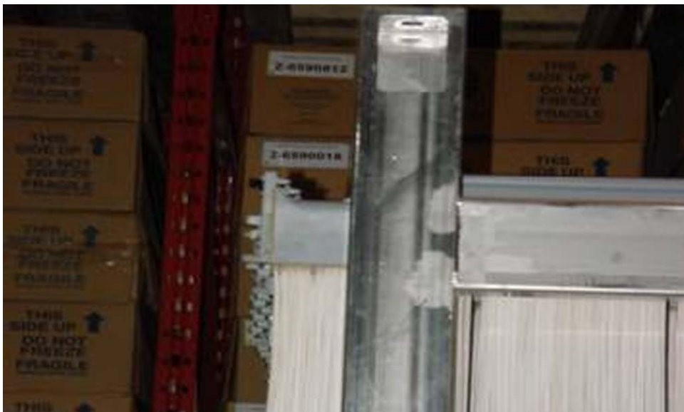
Figure 7.9 - Module Slid Out of Cassette
