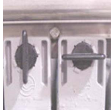
Figure 5.30 - Unlocked Module Key
