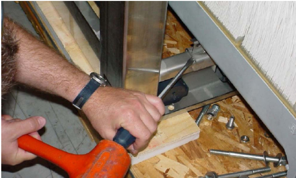
Figure 7.10 - Adjusting the Front Bottom Beam
