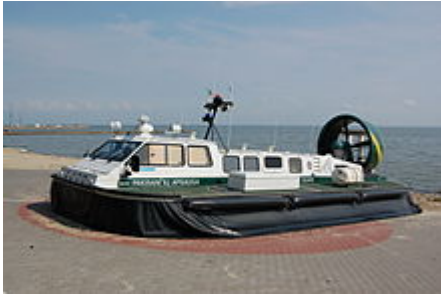
A Lithuanian Coast Guard hovercraft with engine off and skirt deflated
