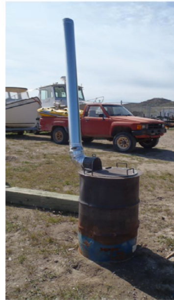
Figure 4 – Modified Burn Barrel
