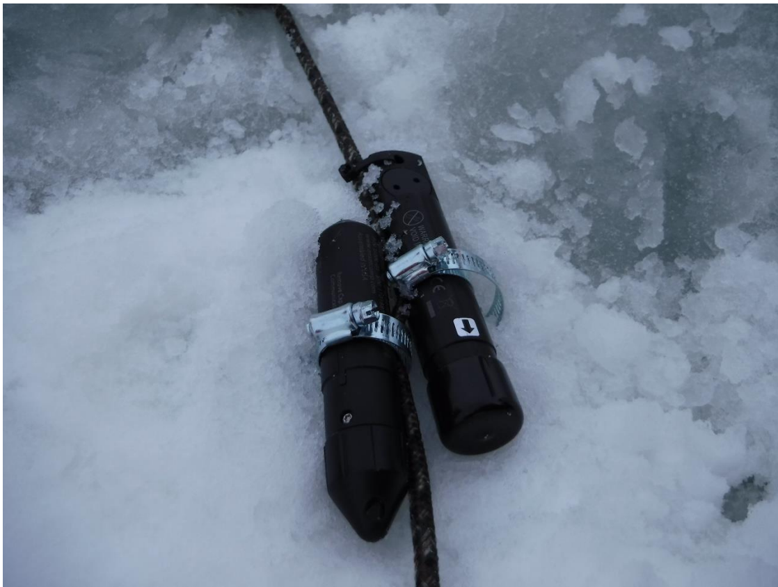
Above photograph of conductivity and temperature probes attached to a rope using hose clamps, ready to be lowered into the water for the winter season.
