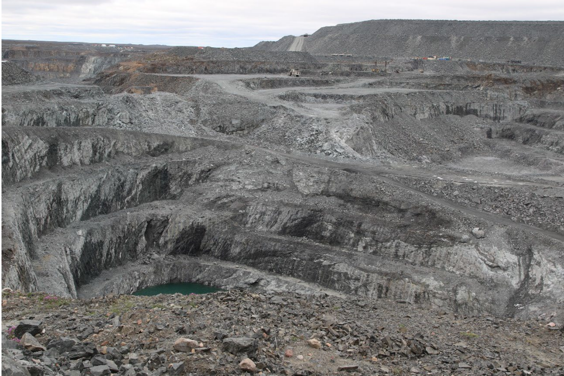
Photo 51: IVR Pit – temporary storage of saline fluid as described in the 2023 modification.
