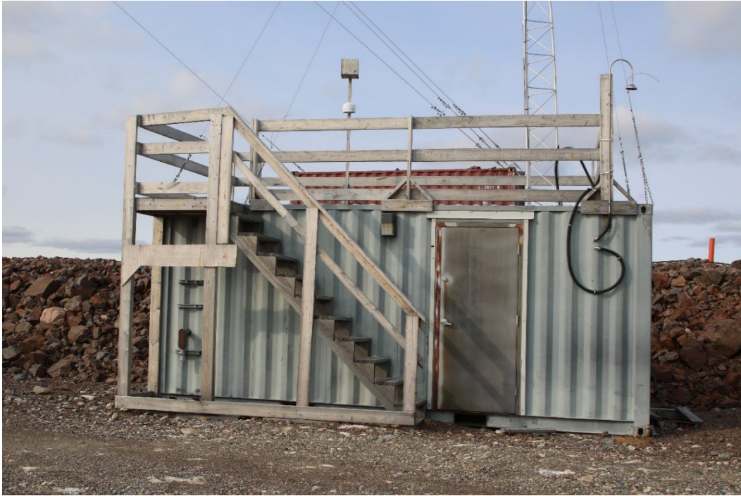
Photo 41: Seacan housing the active NO 2 monitoring equipment with a Passive NO 2 monitor on the roof.
