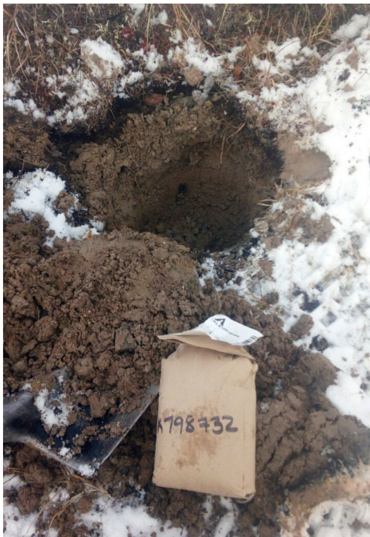
Figure 5: Typical Infill Till Sampling Station
