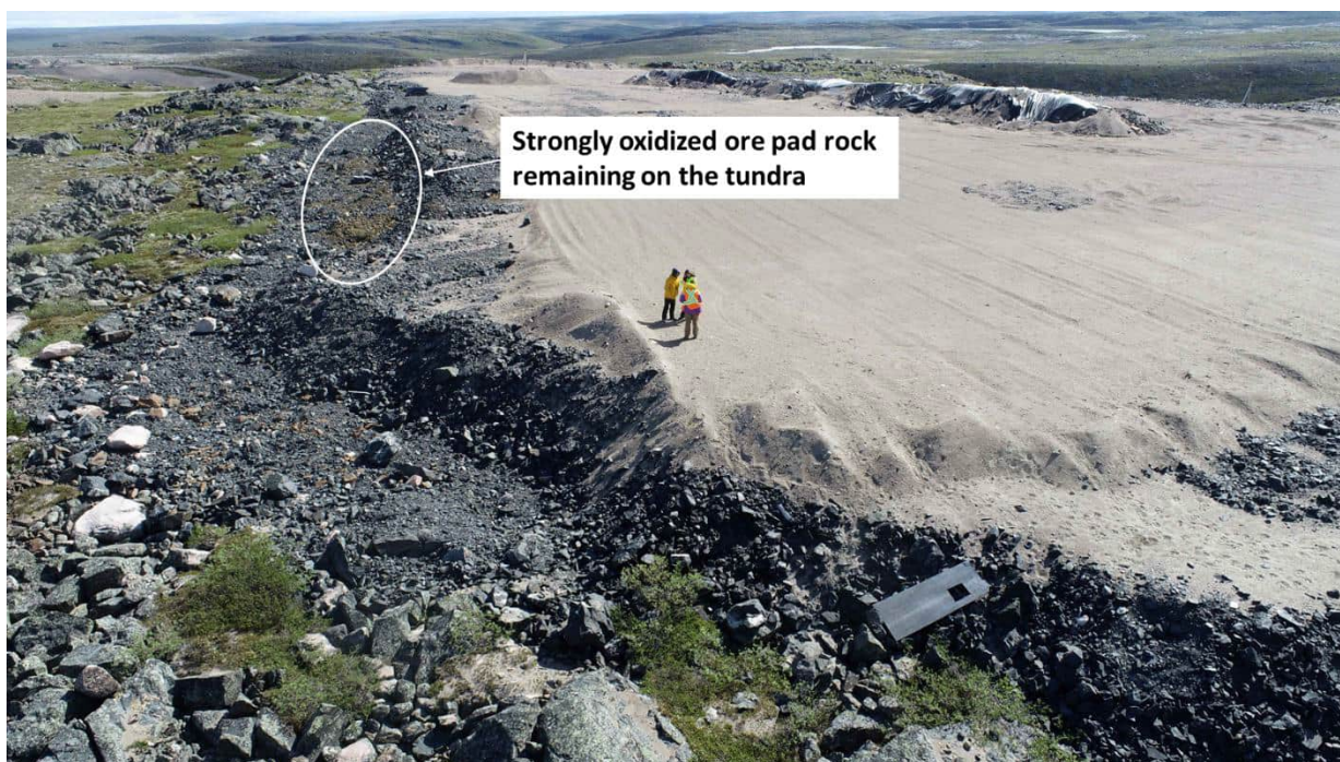
Figure 5-16. Arial View of the North Edge of the Ore Pad Prior to Remediation in August 2024 (Looking East).
