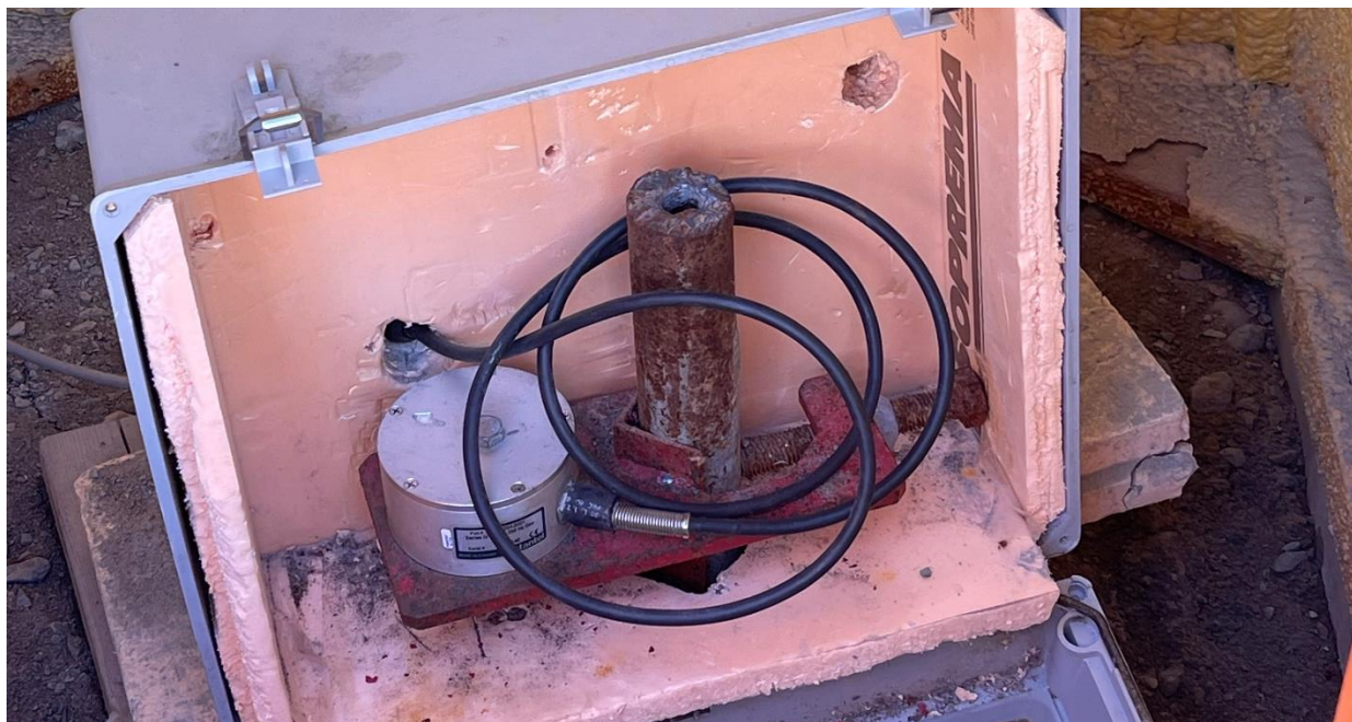
Photo 40: Blast monitoring station.
