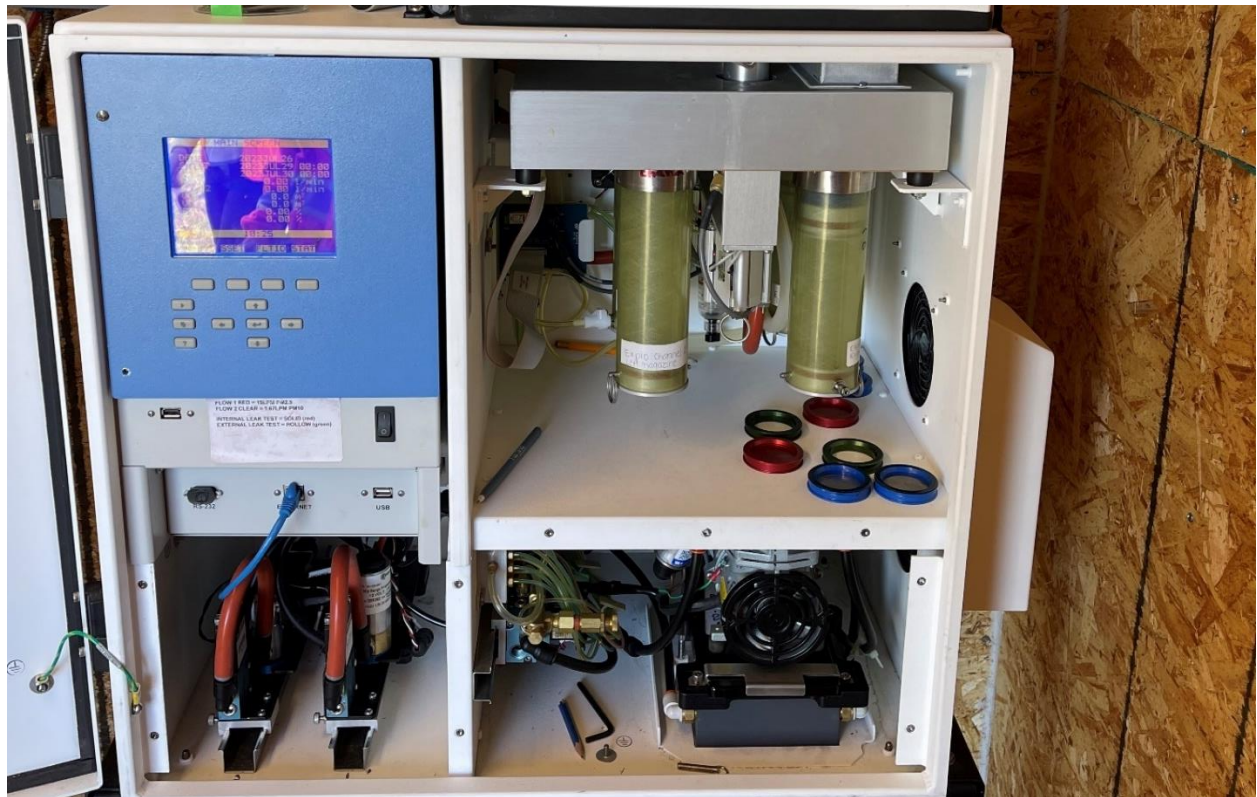
Photo 38: Partisol active air quality monitor.
