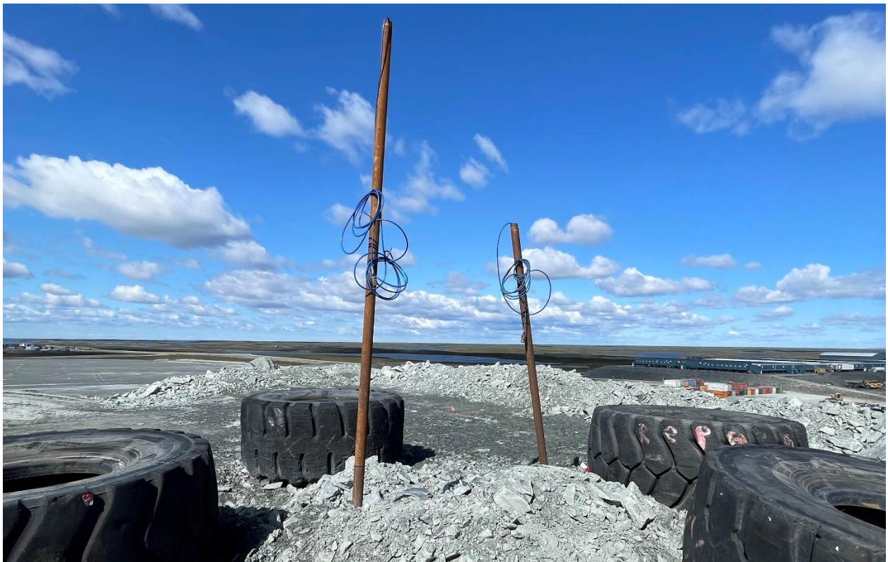
Photo 30: Ground temperature cables are placed in the tailings.
