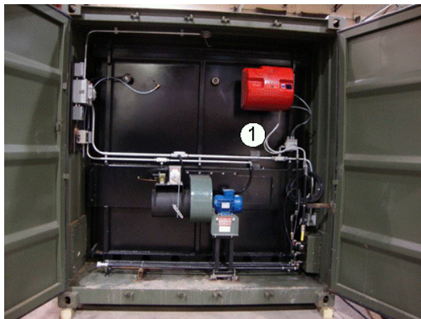
Primary Chamber Burner Flexible lines
