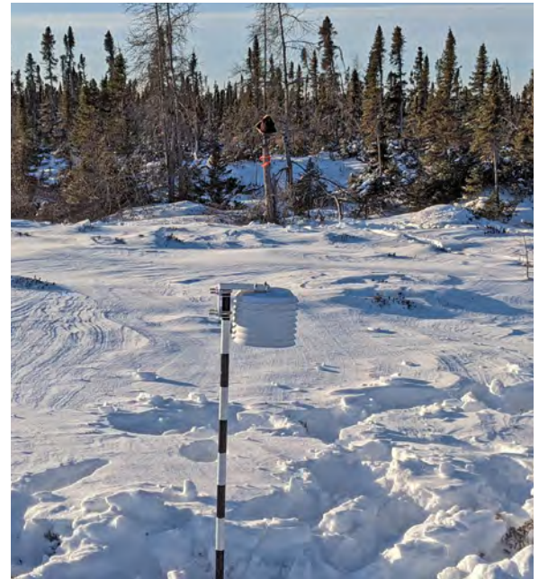
AIR TEMPERATURE AND HUMIDITY SENSOR INSTALLED NEAR KHFL005, (SEE MAP 7 NEXT PAGE) WITH TRAIL CAMERA IN THE BACKGROUND
