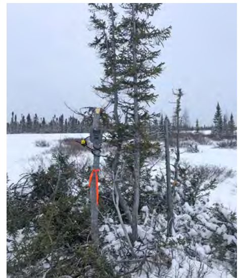
TRAIL CAMERA WITH TREE TOPPED TO REDUCE WIND SWAY
