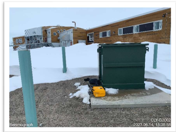
Seismograph Installed Before Each Blast Beside the Cultural Learning Center
