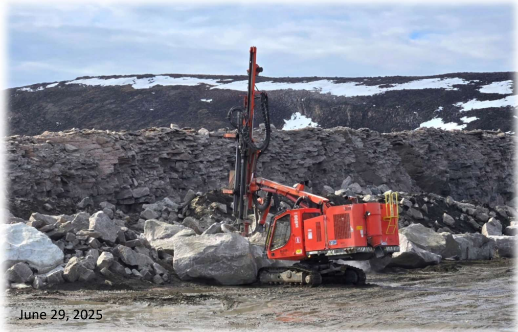
Drilling for blasting oversize rocks
