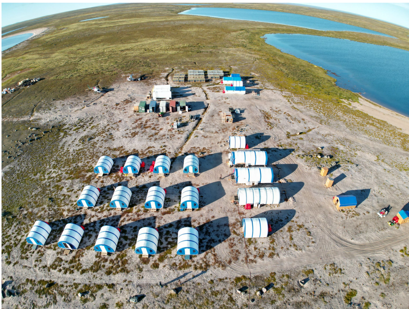
Figure 10-9 Aberdeen Camp built in 2024. Tents in the lower left are sleepers. Large tents in the centre are the kitchen and dry/shower tents. Incinolet toilets and generator shack are to the lower right.
