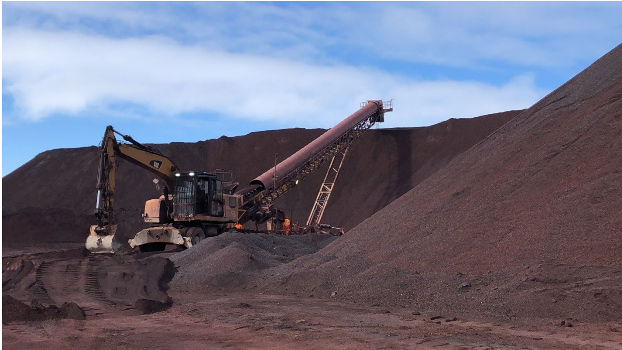
Figure 7 Ore being deposited at stockpiles with luffing stacker (June 2022)
