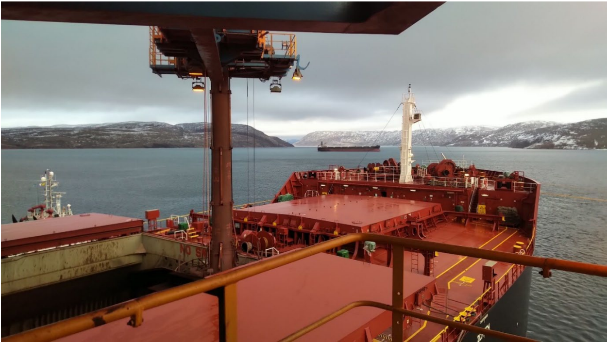
Figure 19 Telescopic chute in cargo hold of ship (height of active loading) (October 2021)
