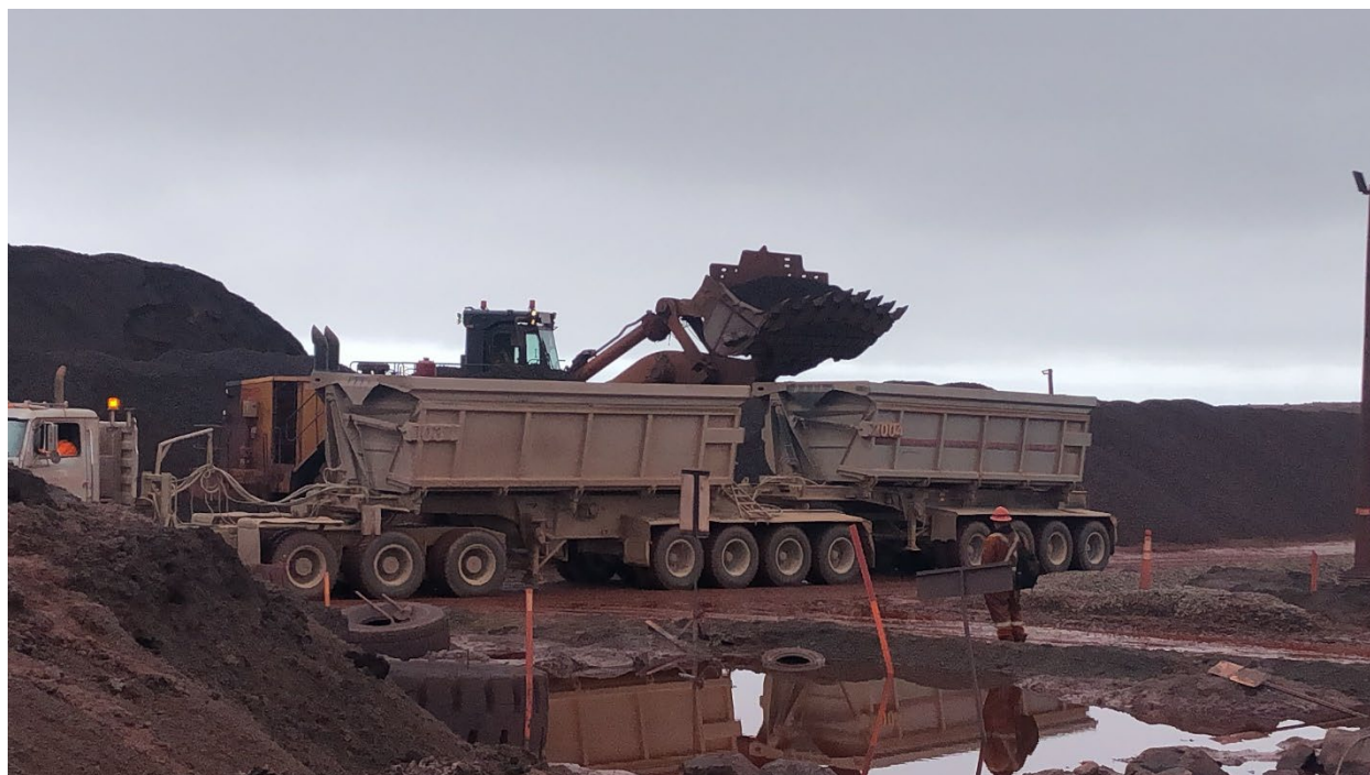
Figure 14 Loading of B-Trains by a FEL (June 2022)
