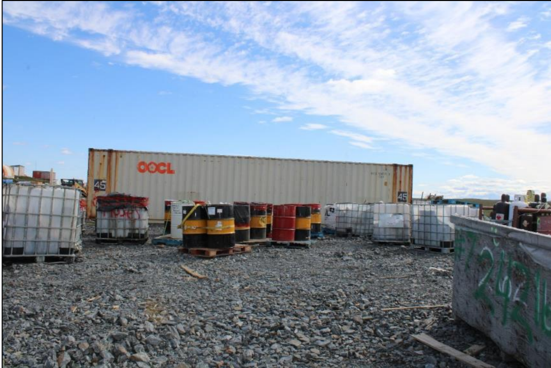
Photo 16: Hazardous Materials Stored outside of lined containment.
