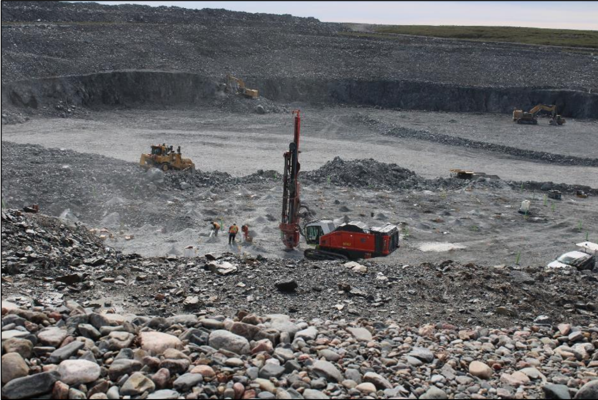
Photo 19: Blasting preparation in Echo Pit.
