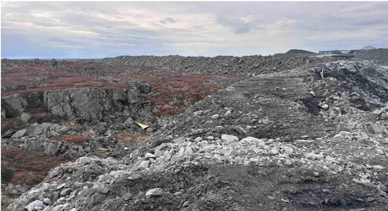
G-226: ROM stockpile SE end – daylighting into tundra
