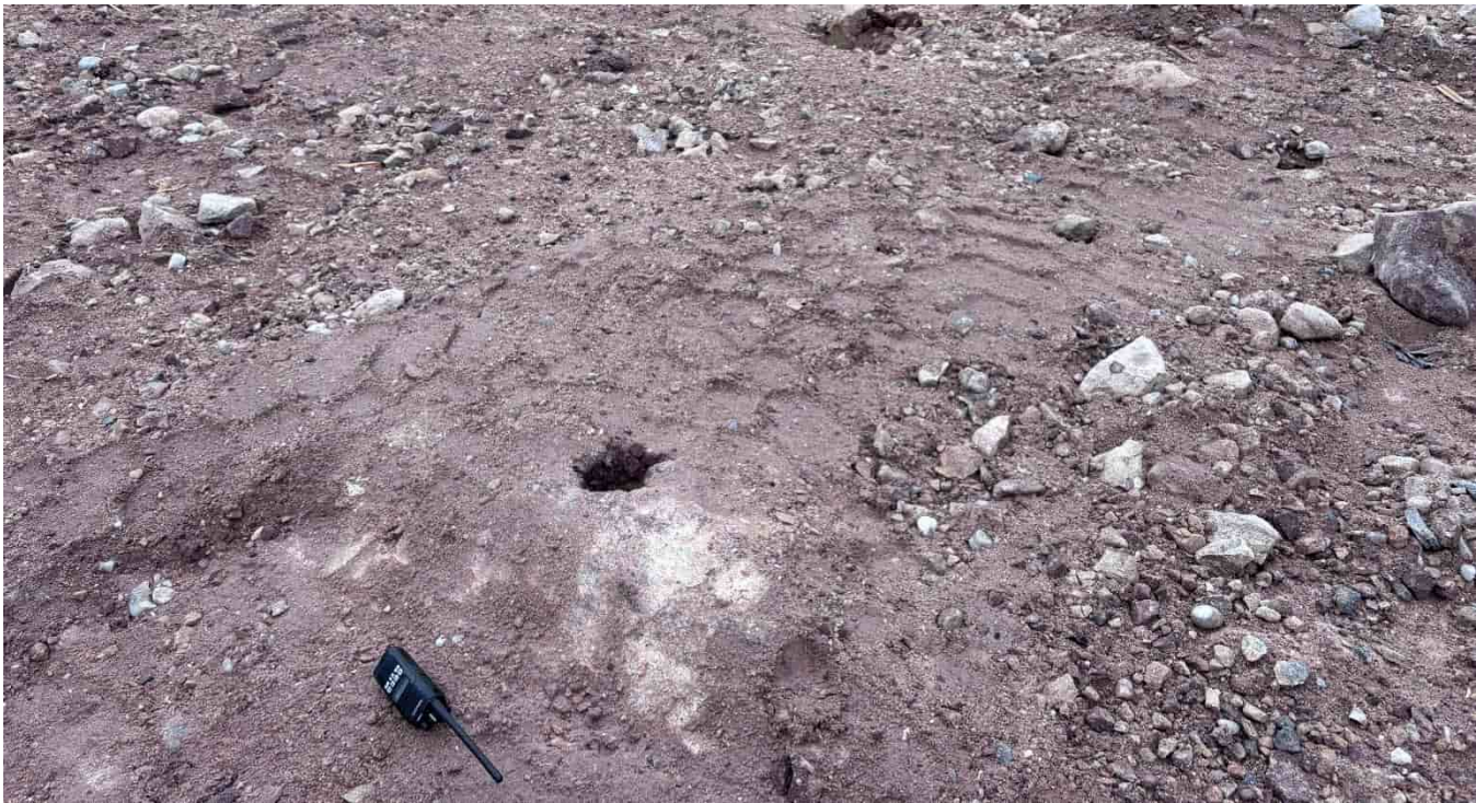
M-220: Holes that were drilled in the area but not blasted
