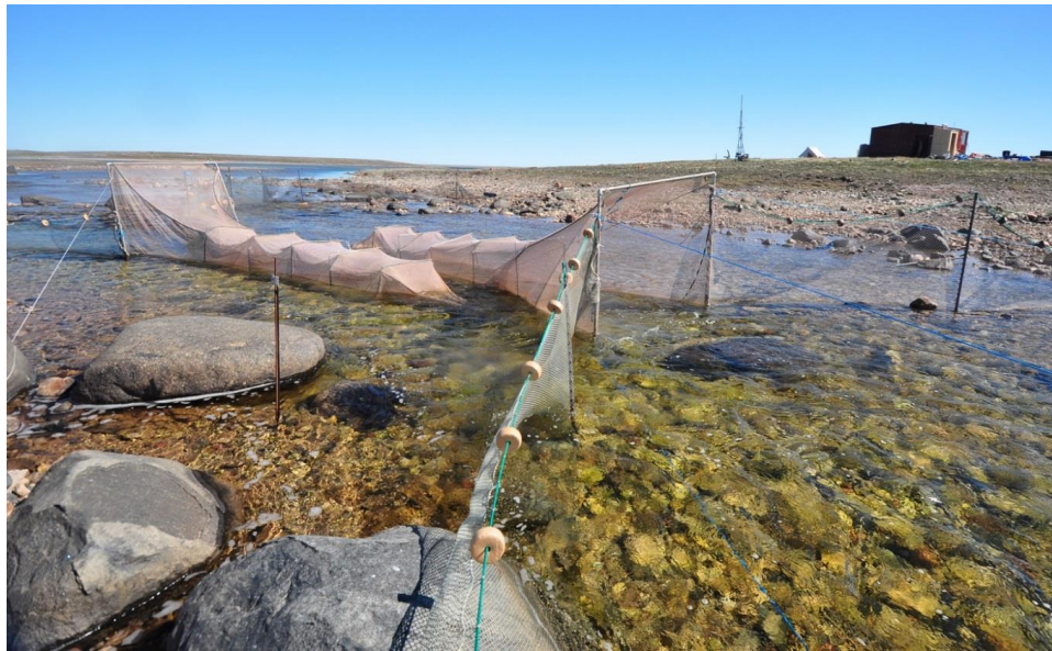
Photo 7.2-1 Two-way Fyke-net trap at mouth of Nulahugyuk Creek, July 2016.
