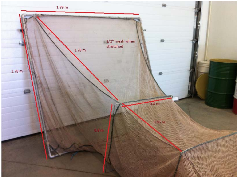
Photo 4: Fyke Net Throat Including Dimensions
