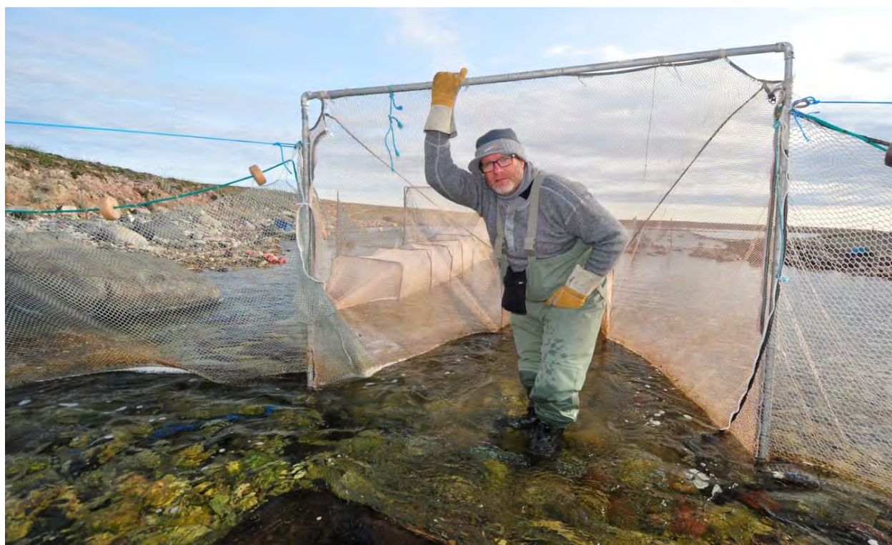
Photo A-2: Downstream fyke-net trap used to capture out-migrating juvenile Arctic Char, 12 July 2016.
