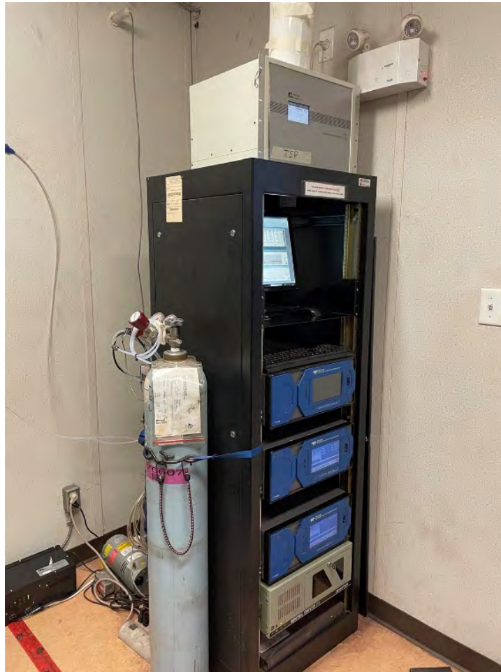
Photo 1.8 The rack-mounted Teledyne T100 (SO 2 ) and T200 (NO x -NO 2 ) continuous gas analyzers at the PSC. The BAM 1020 analyzer for TSP is at the top of the rack.
