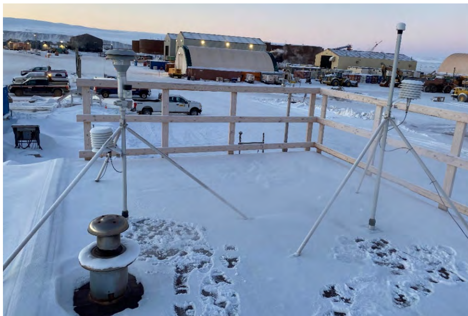
Photo 1.4 The TSP and PM 2.5 roof mount outlets and cutter heads.
