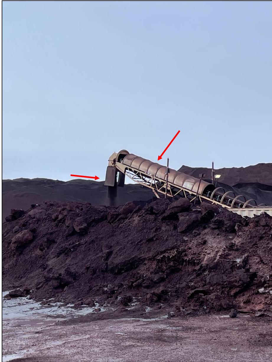
Photo 17: Bellows and Shrouds at the end of the Crusher Conveyor System (Arrows).
