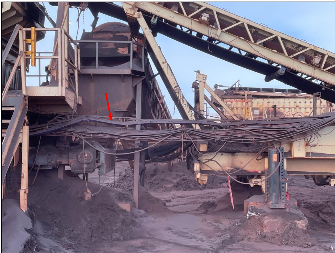
Photo 20: Heat Traced Pipe for Delivery of Dust Suppressant (Arrow).
