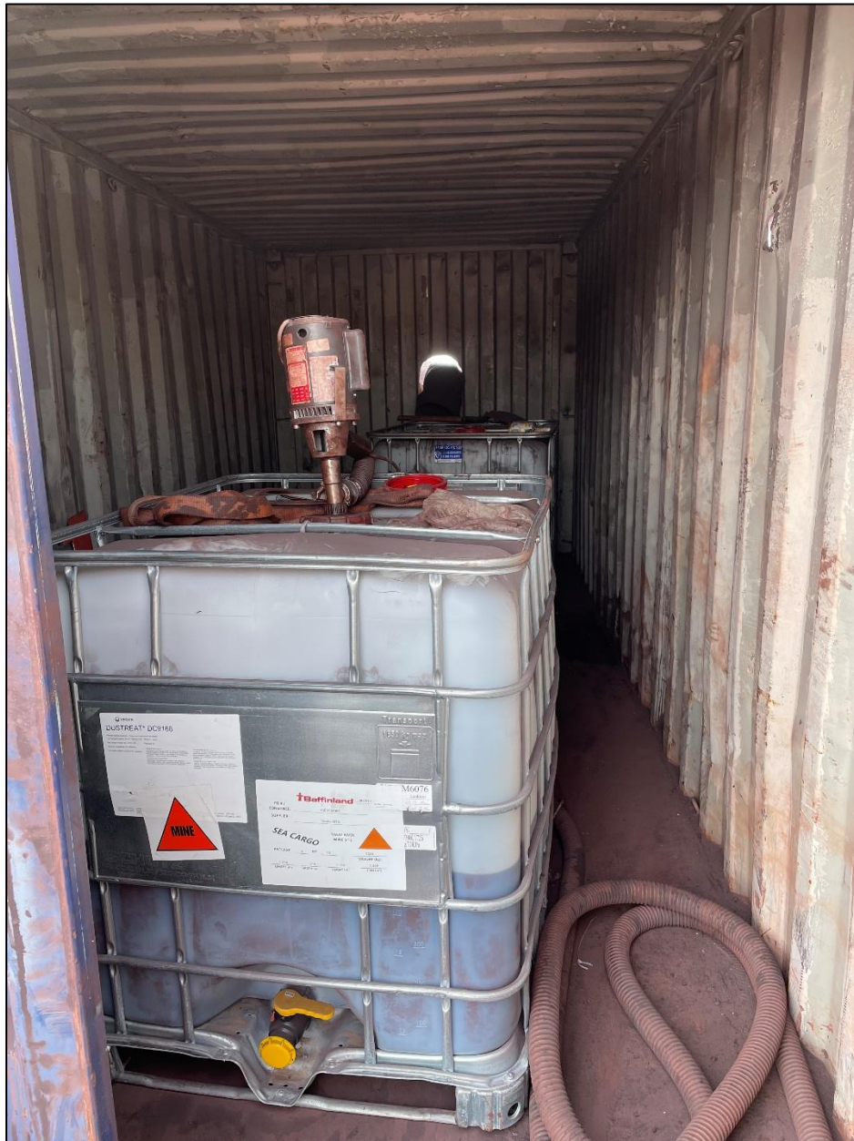
Photo 21: Liquid Dust Suppressant Stored in a Heated Seacan next to the Crusher.
