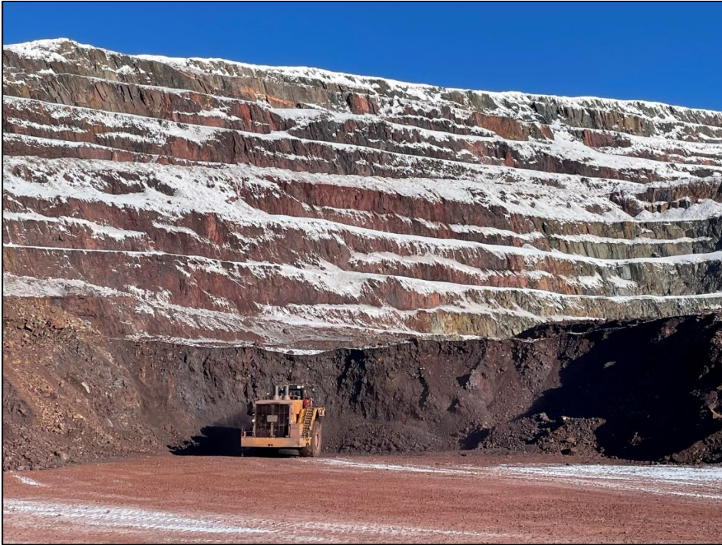
Photo 27: Deposit No. 1 Pit Benches and Working Face.
