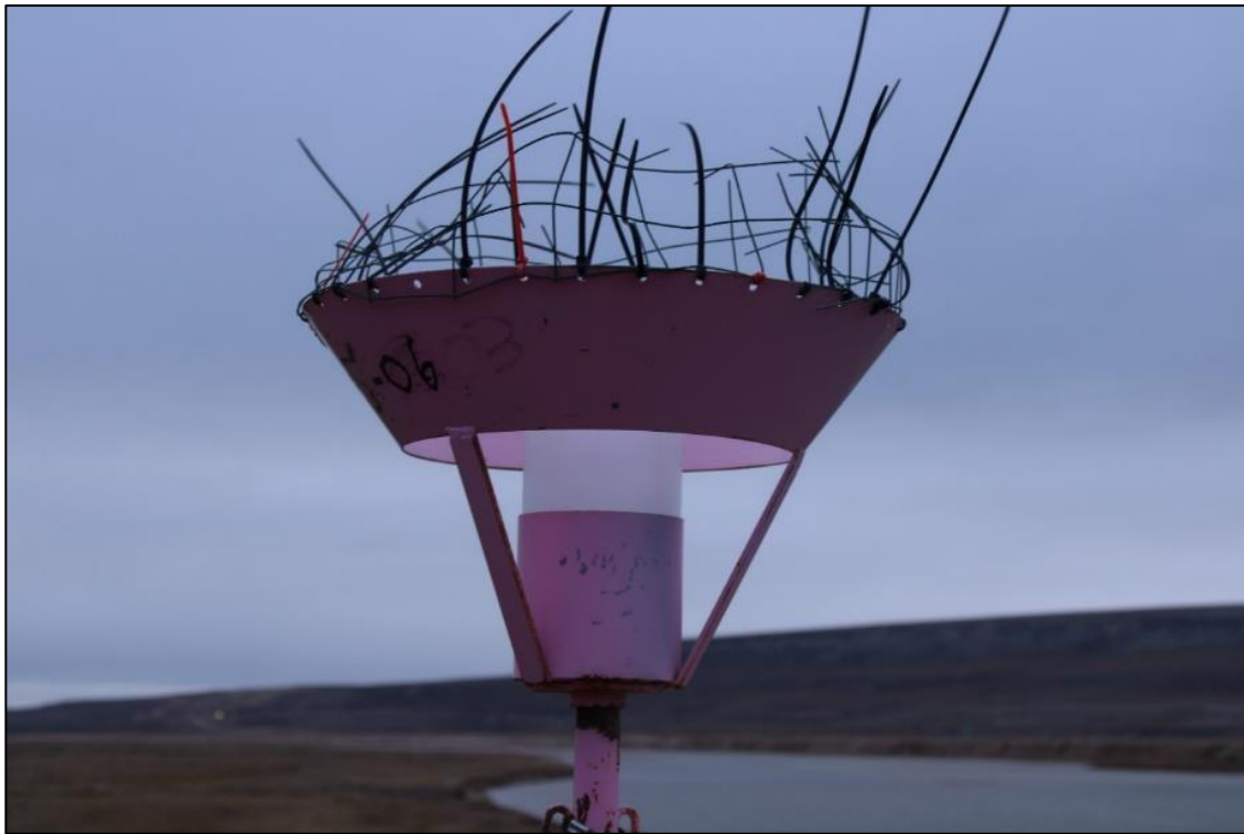
Photo 47: Close-up of Passive Dust Sampler Container.
