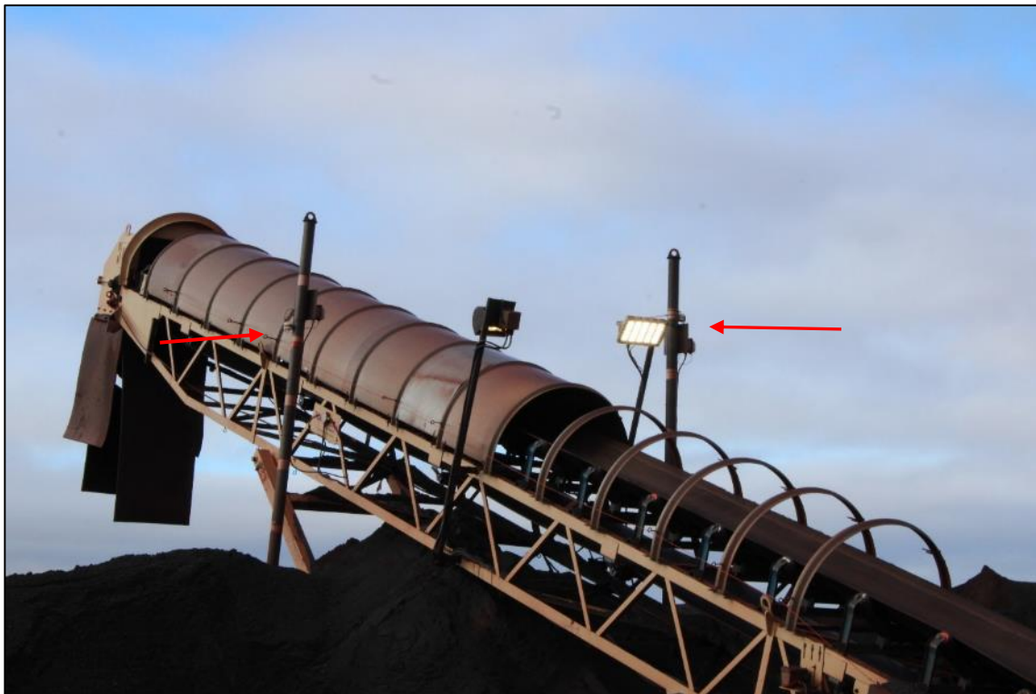
Photo 10: Hoods and Shrouds along the Crusher Conveyor with Active Air Sampler to Measure Dust Production (Arrows pointing to air samplers).
