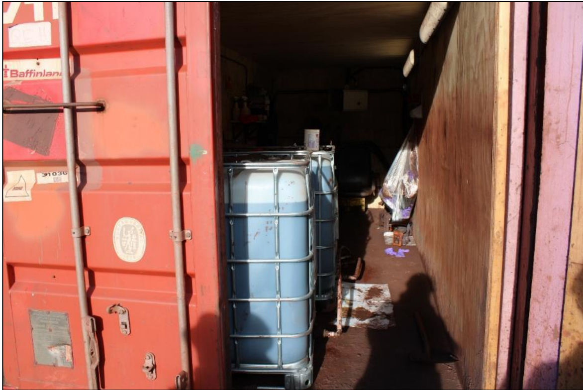
Photo 13: Liquid Dust Suppressant Stored in a Heated seacan next to the Crusher.
