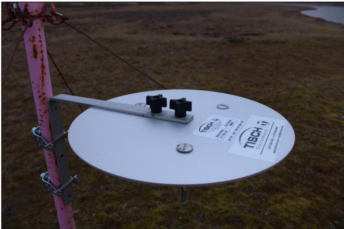
Photo 48: New "Disc Style" Passive Dust Sampler from NRCan Study.
