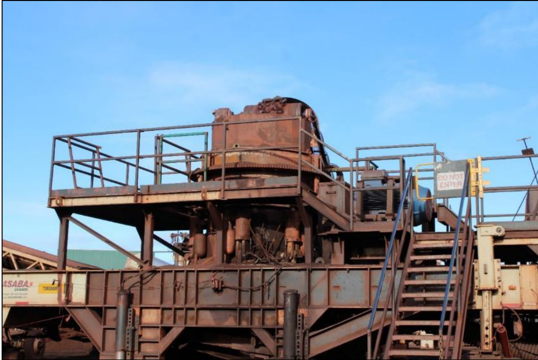
Photo 11: Cone Crusher along the Conveyor System at the Crusher Facility.
