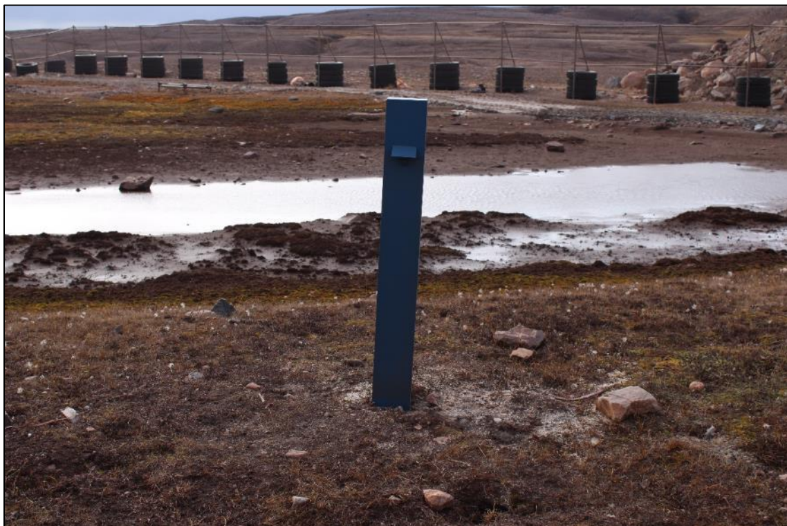
Photo 32: Ground Water Monitoring Station in Landfill.
