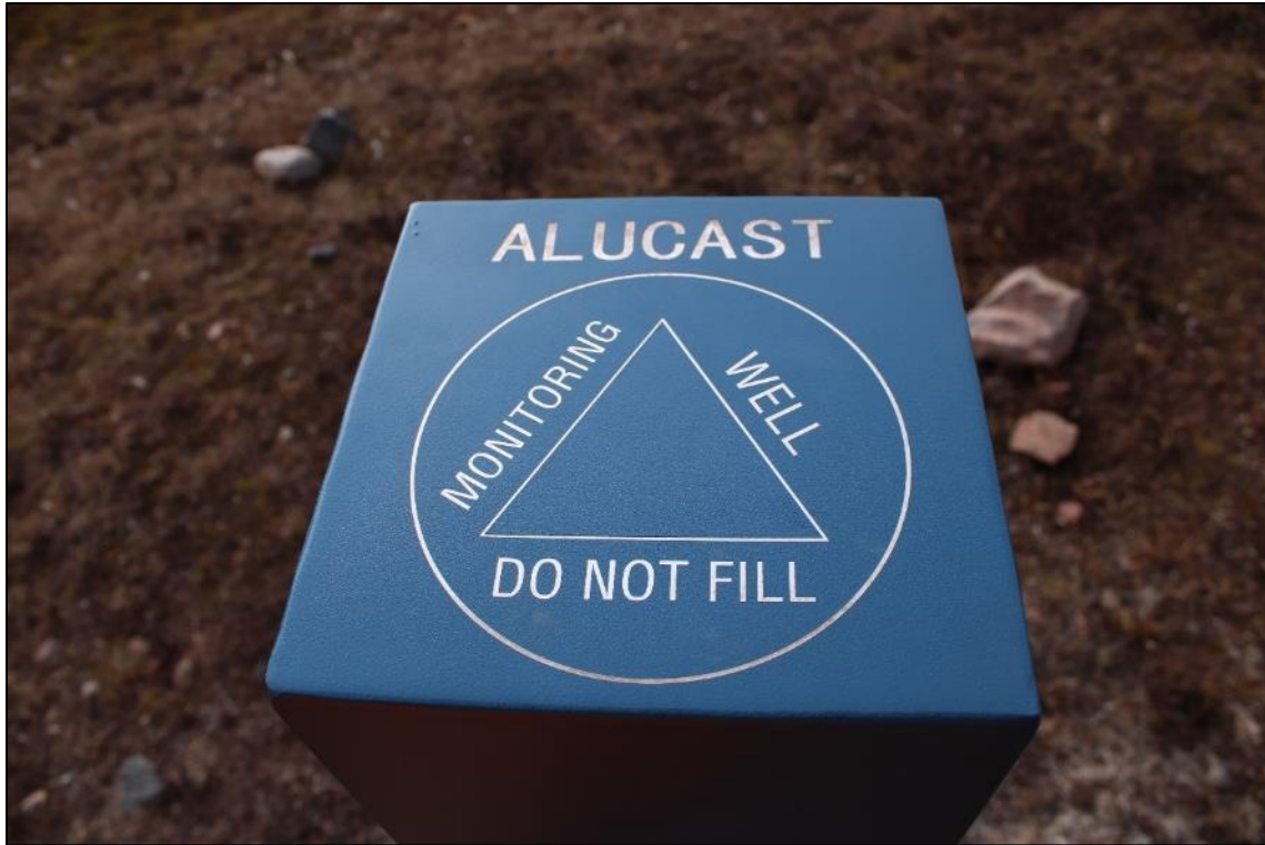
Photo 33: Ground Water Monitoring Well Cover.
