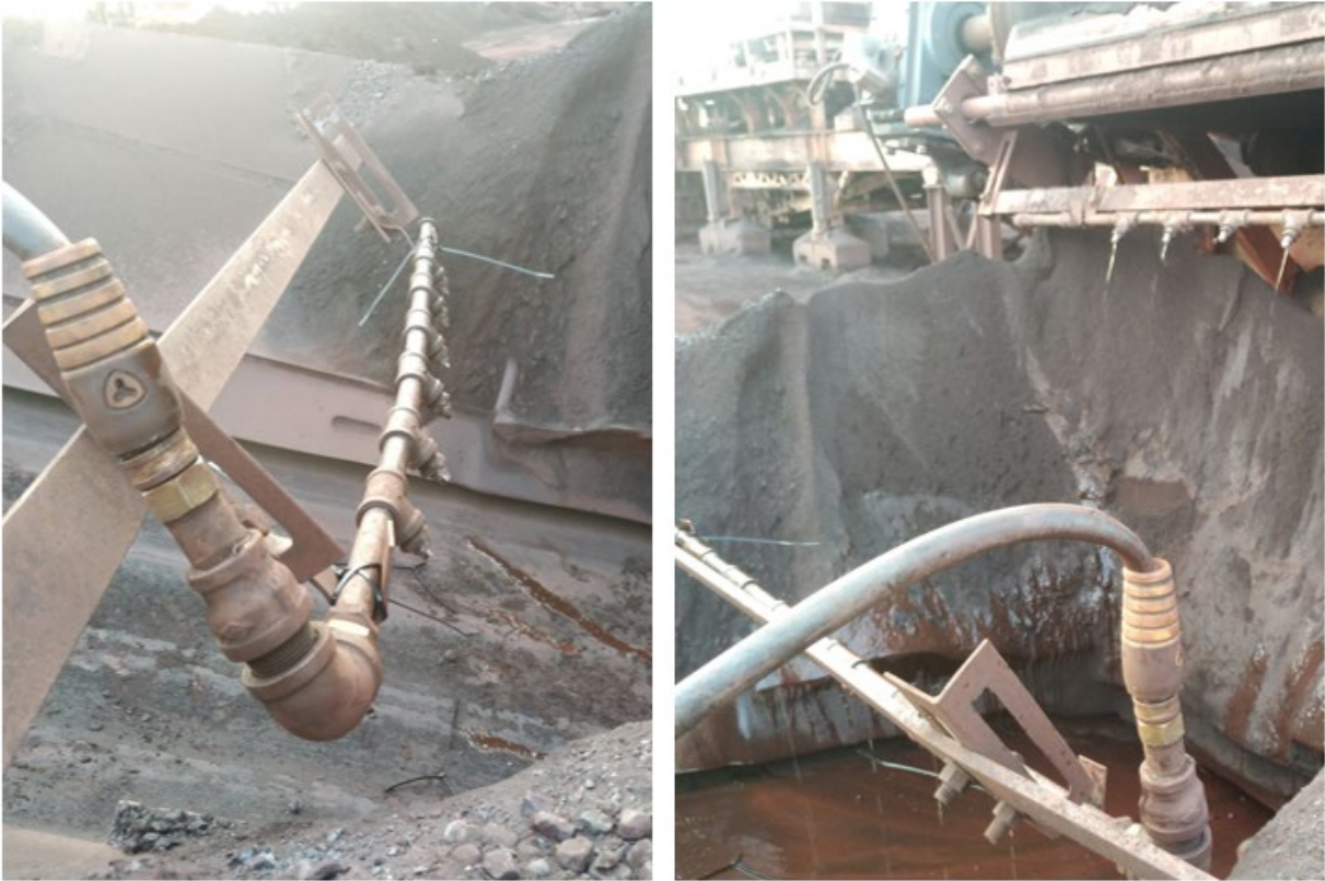
Figure 8 Visual of Crusher Dust Suppressant Nozzles at Crusher Line C trial (provided by Baffinland, January 2025)
