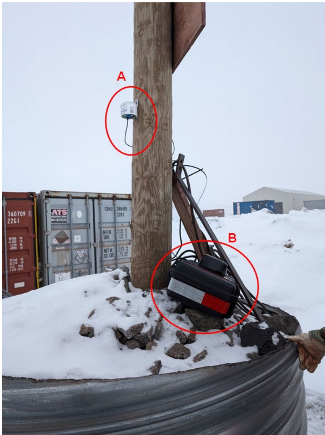
Figure 9 PurpleAir Monitor (labelled A) near airstrip connected to device (labelled B) that shares data to Baffinland on demand (April 2024)
