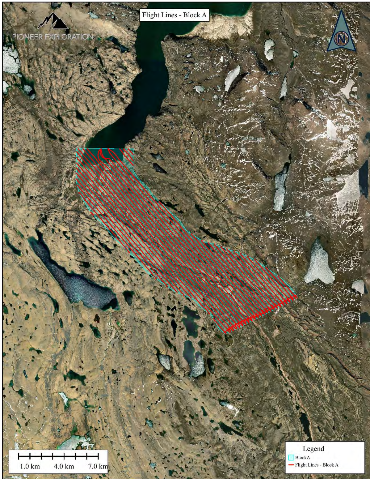
Figure 2a: LiDAR Survey Block A flight line coverage.
