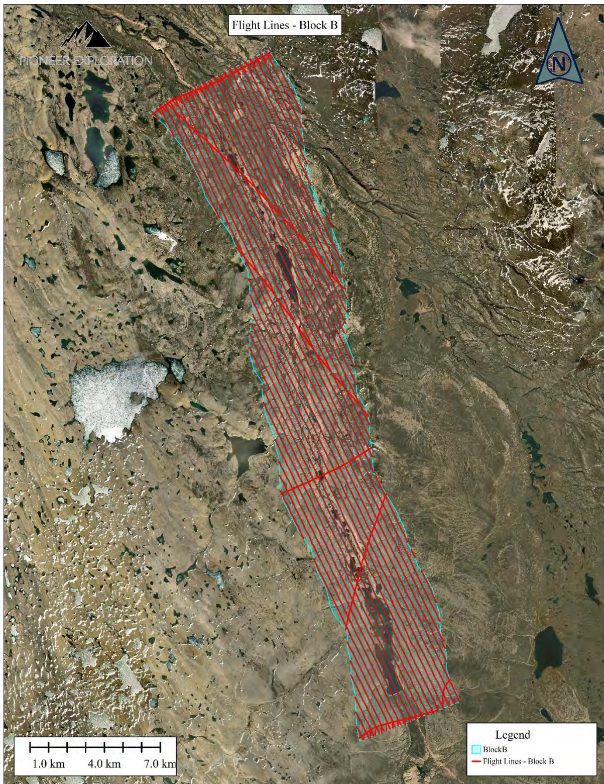
Figure 3b: LiDAR Survey Block B flight line coverage.
