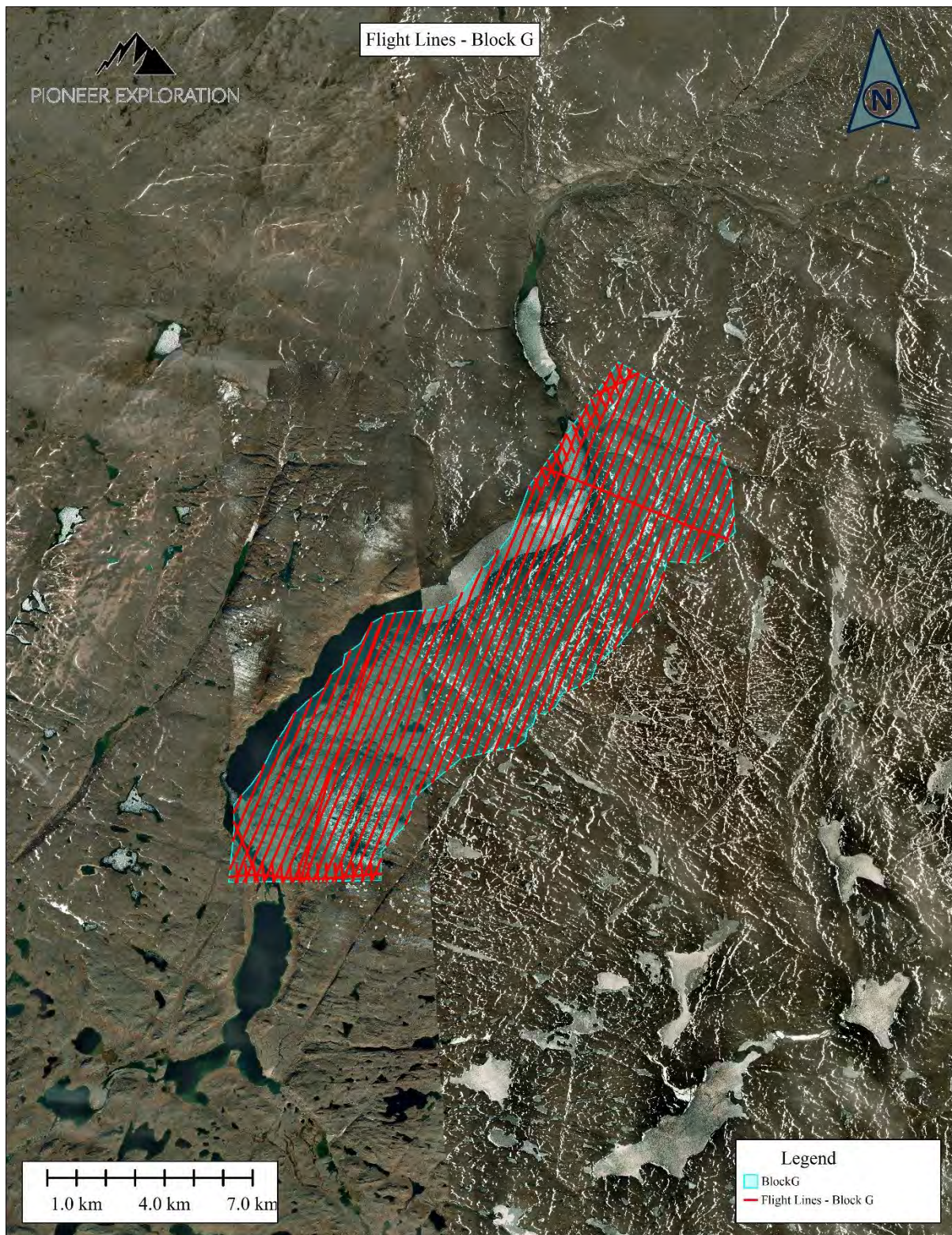
Figure 8g: LiDAR Survey Block G flight line coverage.
