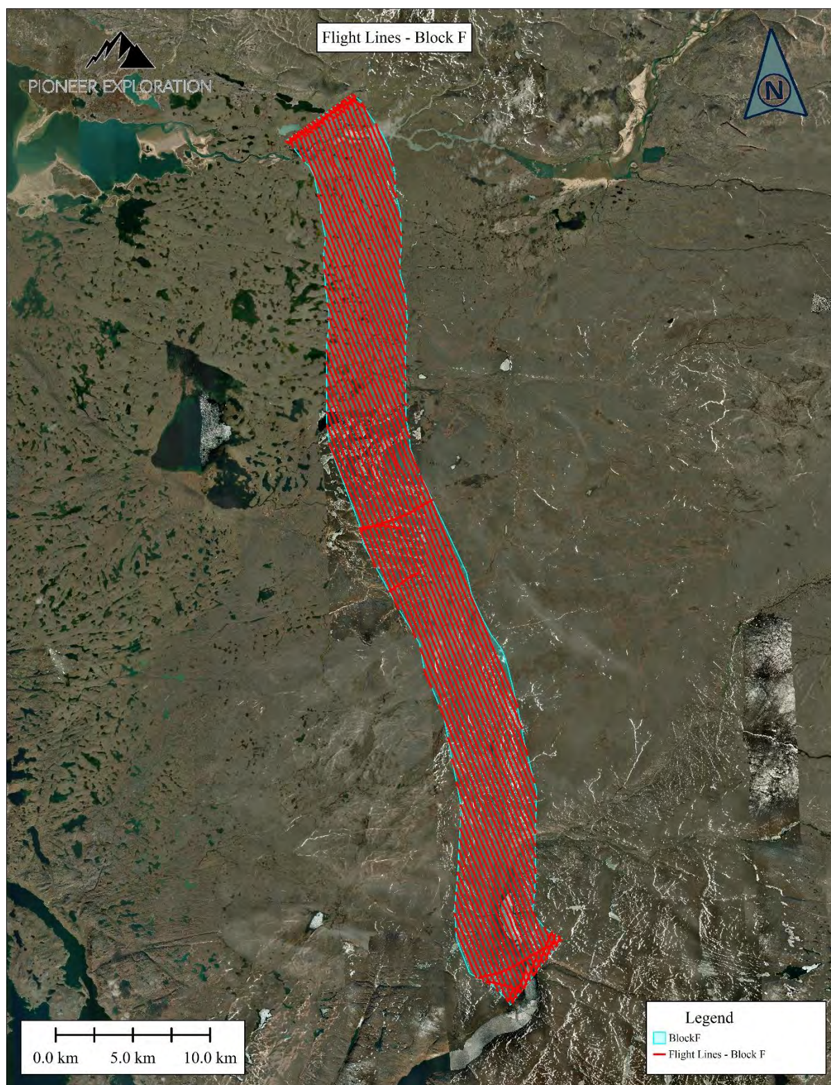
Figure 7f: LiDAR Survey Block F flight line coverage.
