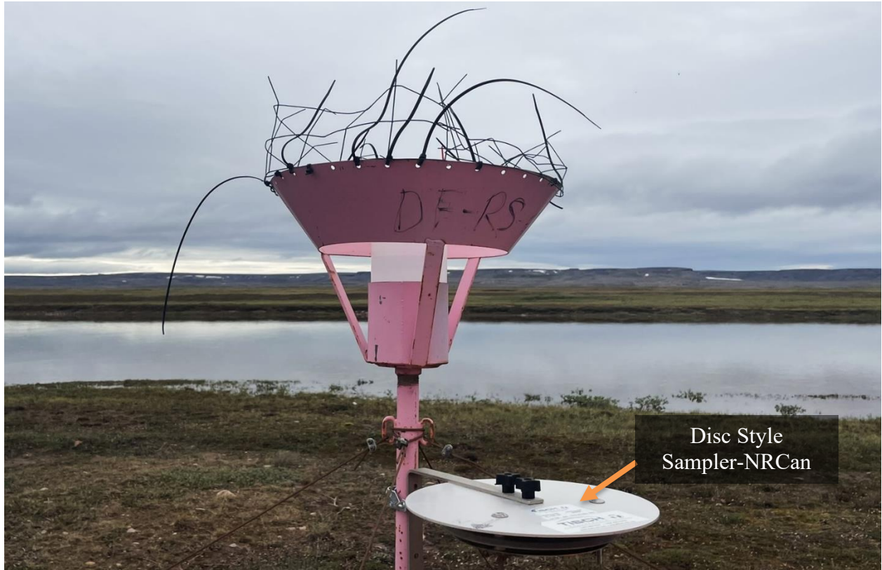
Photo 54: Passive dust sampler and "Disc Style" passive dust sampler from NRCAN Study at KM 79.5
