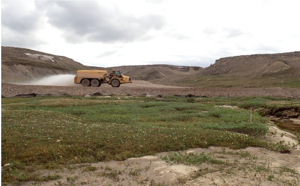
Photo 10: Water Truck Applying Dust Suppression – July 2025
