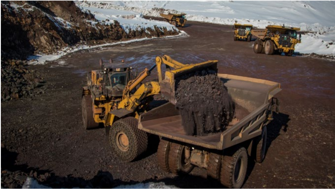
Photo 2: Iron Ore Being Loaded onto Mine Haul Trucks
