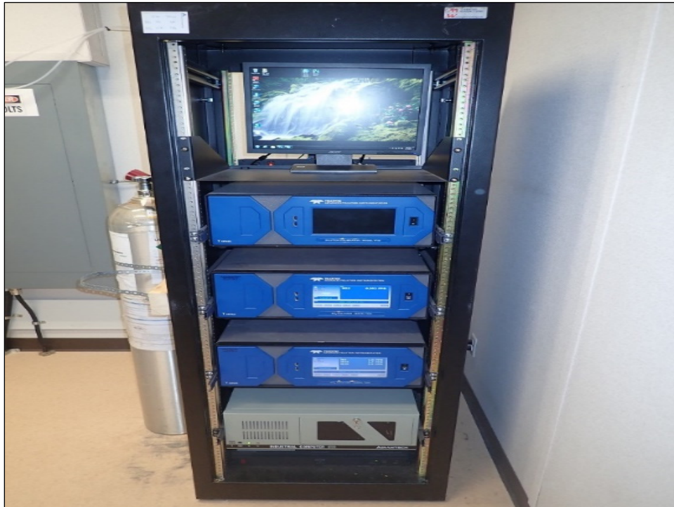
Photo 3.1-1 Rack-mounted Teledyne T100 (SO 2 ) and T200 (NO x -NO 2 ) continuous gas analyzers at the Mine Site Complex ambient air quality station.
