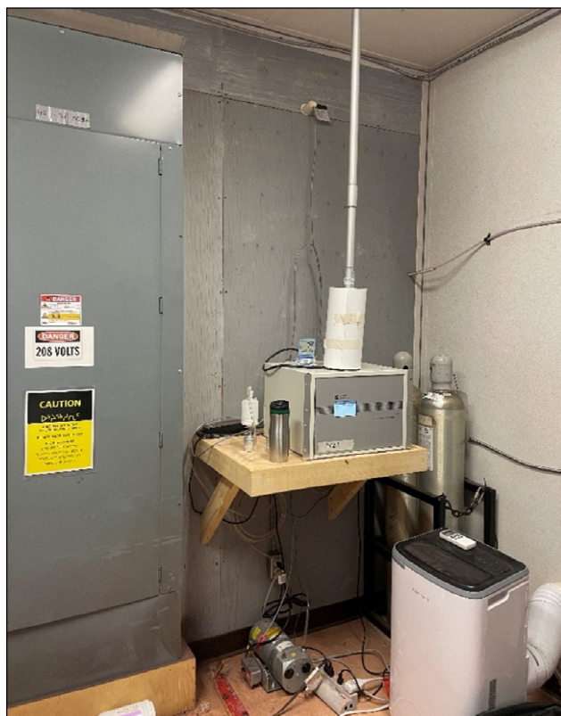
Photo 3.1-4 PM 2.5 BAM 1020 analyzer at the Mine Site Complex ambient air quality station.
