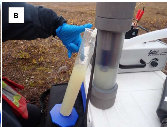
Photo A-2: A) Standpipe well LF-KP23-09 (August 25, 2025), B) Measuring volume of purged water.
