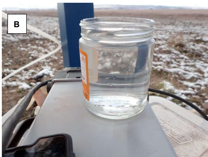
Photo A-48: Well development at MS-HWB-25-03 (August 29, 2025) – A) Standpipe well MS-HWB-25-03, B) Water clarity after 5 well volumes, C) Water clarity after 10 well volumes.
