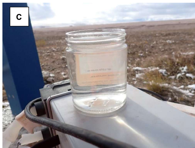
Photo A-48: Well development at MS-HWB-25-03 (August 29, 2025) – A) Standpipe well MS-HWB-25-03, B) Water clarity after 5 well volumes, C) Water clarity after 10 well volumes.
