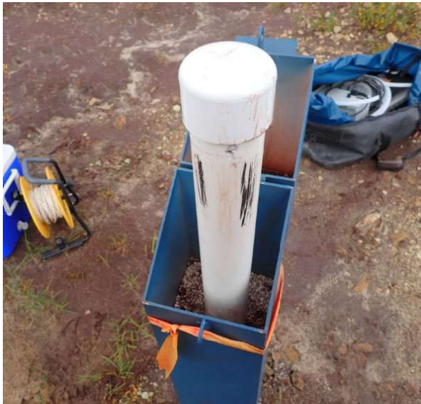
LF-KP22-05 well casing and monument.
