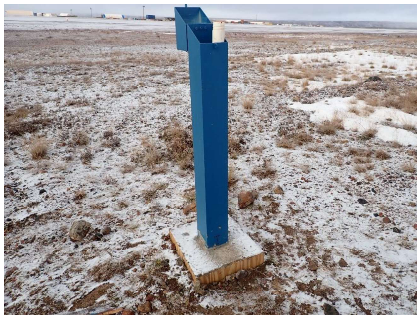
Photo A-46: Standpipe well MS-HWB-25-03 (September 4, 2025) – Slug test was completed at the well location.
