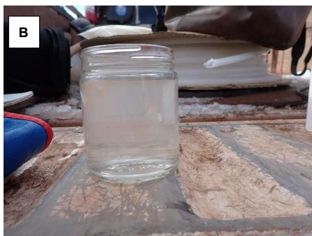
Photo A-47: Well development at MS-HWB-25-01 (August 29, 2025) – A) Standpipe well MS-HWB-25-01, B) Water clarity after 2 well volumes, C) Water clarity after 10 well volumes.
