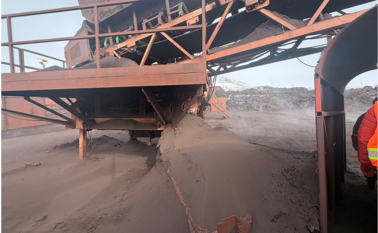
Photo 16: Accumulation of fine ore dust beneath crusher A conveyors, likely due to vibration-induced spillage
