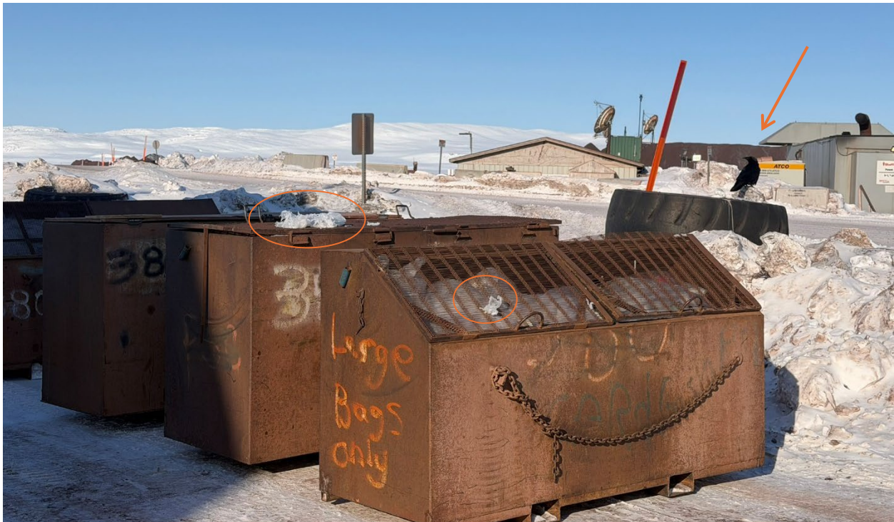
Photo 92: Domestic waste dumpsters adjacent to the incinerator building with mesh-style lids; a raven accessing waste through the openings
