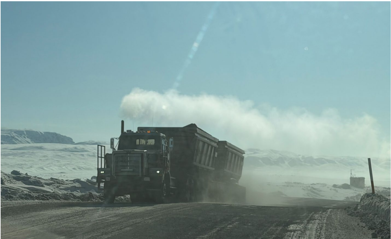
Photo 50: Ore haul truck transporting ore to Milne Port, with fugitive dust generation from tire-road interaction
