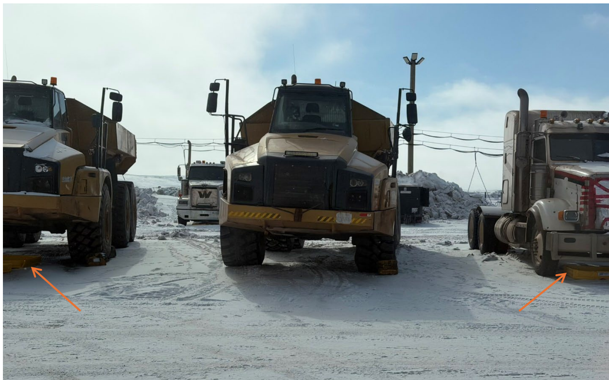
Photo 33: Vehicle and equipment laydown at site services shop, with spill trays observed
