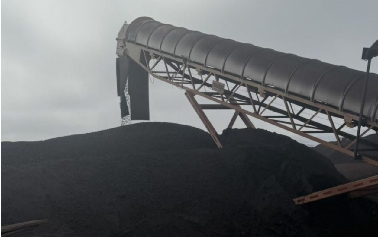
Photo 18: Crusher B outlet showing discharge of coarse, lump ore with no visible dust
