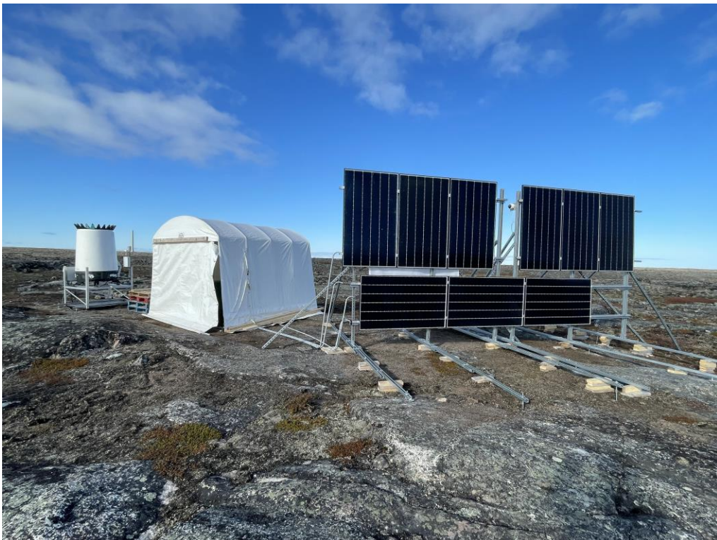
Figure 3. Full setup of the equipment. The SoDAR on the left, the white tent that houses the brains and the backup power supply in the middle, and the solar array that provides the primary source of power on the right.
