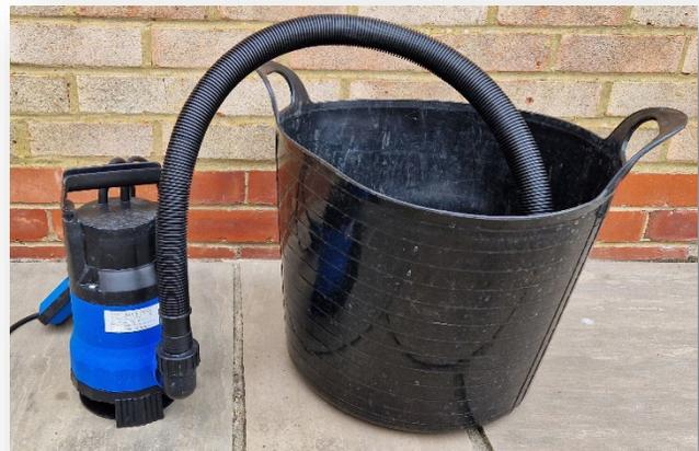
For cold room testing a simple water container will be used, such as the bucket shown (Dims: 490  $\varnothing$  x 360mm, 42 litre)
