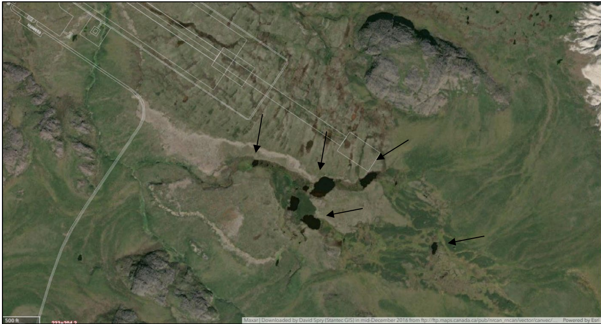
Figure 4.17 Possible thermokarst features (indicated by the black arrows) including depressions and ponds in marine soils next to the aerodrome site.
