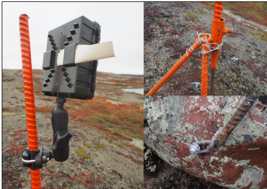
Photo 4.1 Components of a rebar camera tripod mount including RAM© mount (left), wired connection points (top right), and concrete wedge anchors (bottom right).
