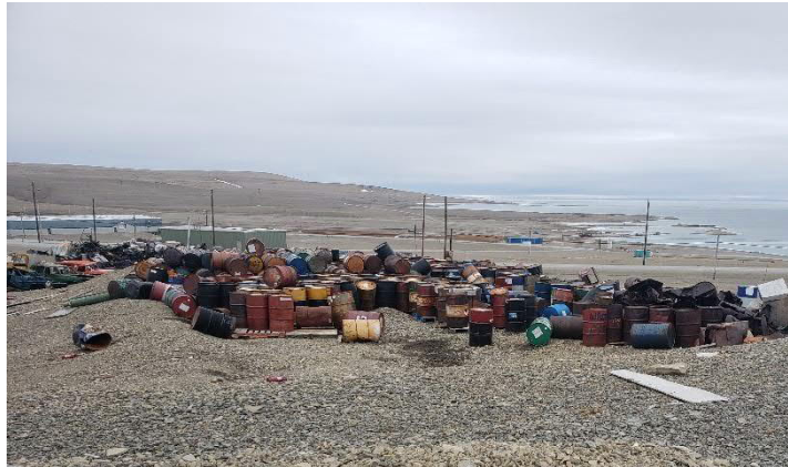
Photo 20: Staining visible near waste oil barrels at the drop-off site
